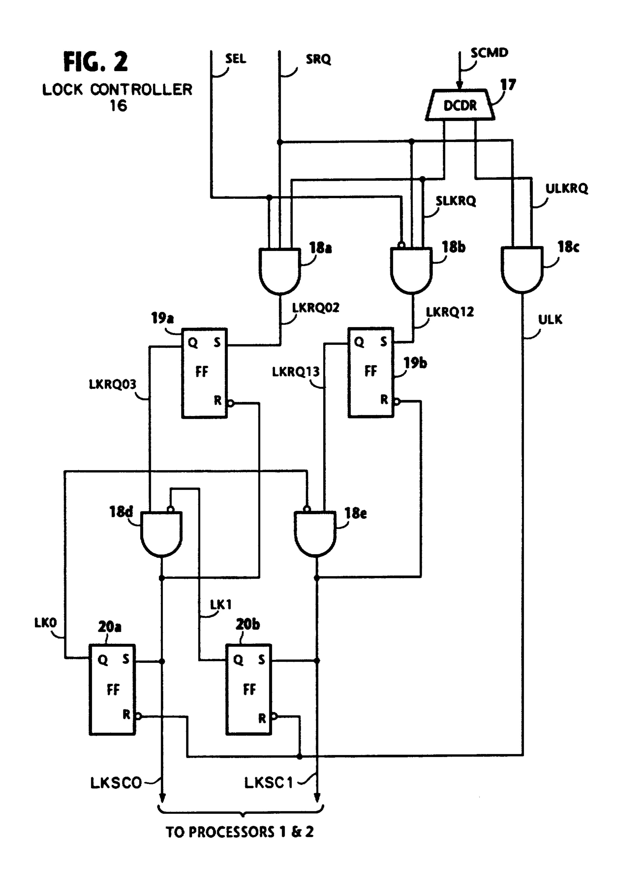
MULTIPROCESSOR SYSTEM INCLUDING AN EXCLUSIVE ACCESS CONTROLLER WITH LOCK REQUEST HOLDING AND GRANT CIRCUITS
