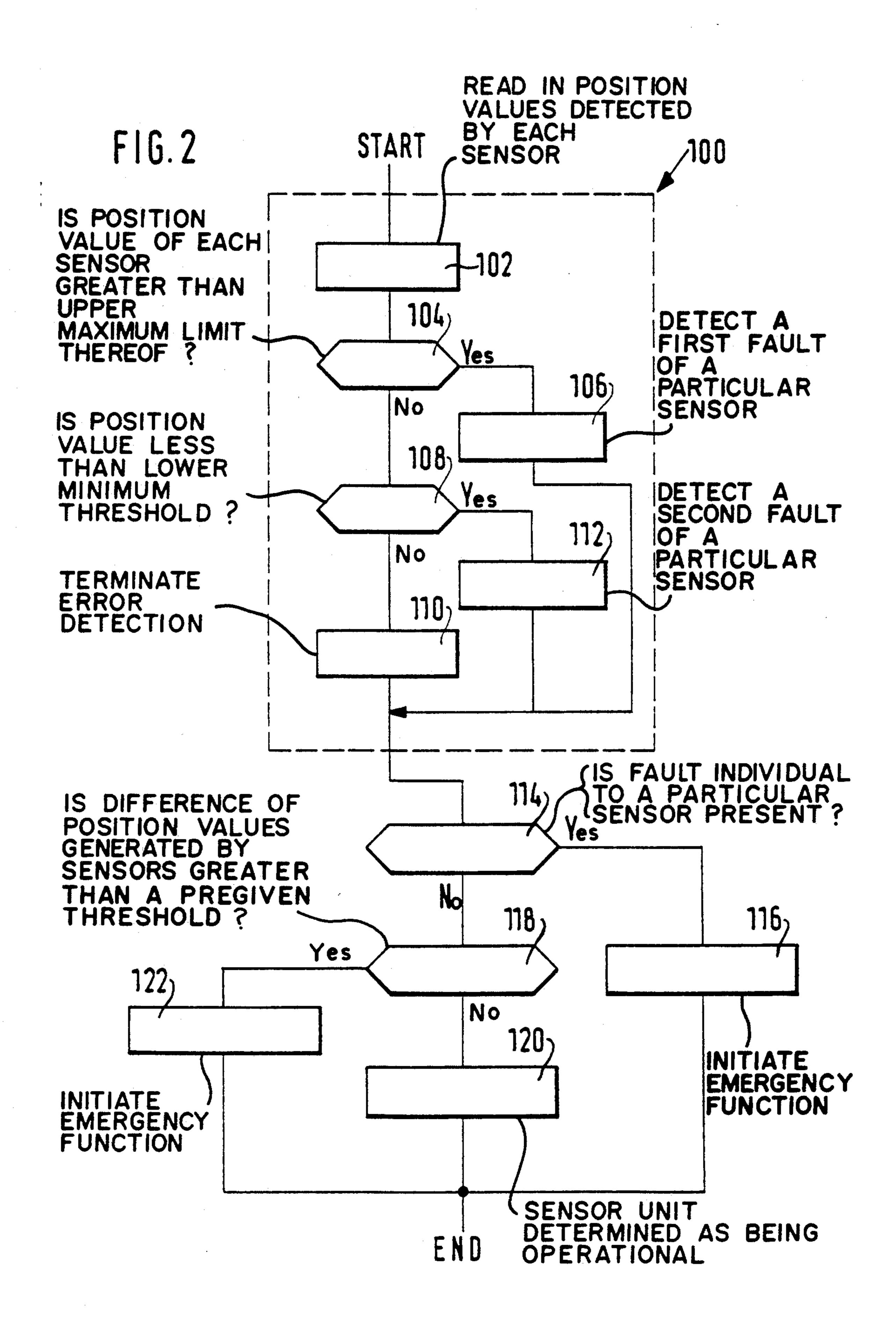
METHOD AND ARRANGEMENT FOR CONTROLLING AN INTERNAL COMBUSTION ENGINE WITH A DETECTING DEVICE UTILIZING TWO SENSORS FOR GENERATING SIGNALS WHICH CHANGE IN MUTUALLY **OPPOSITE DIRECTIONS**
