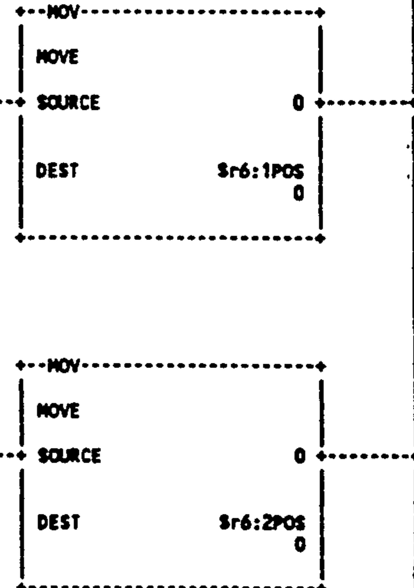
Sr006:001 ... CANISTER 1 BURNOUT DAMPER SEQUENCER
