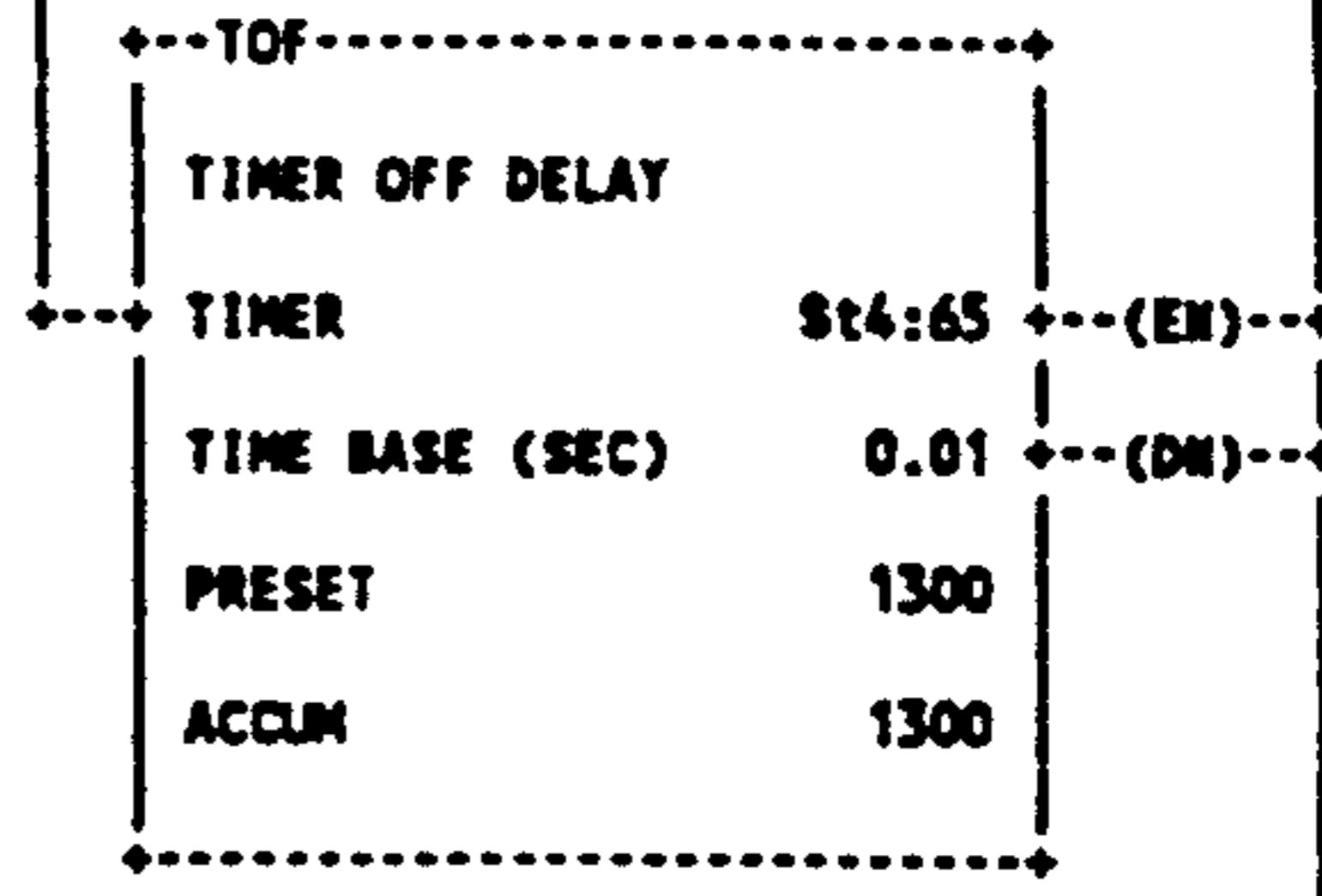
St004:064 ... CANISTR 5 INLET DAMPER DELAY CLOSE
