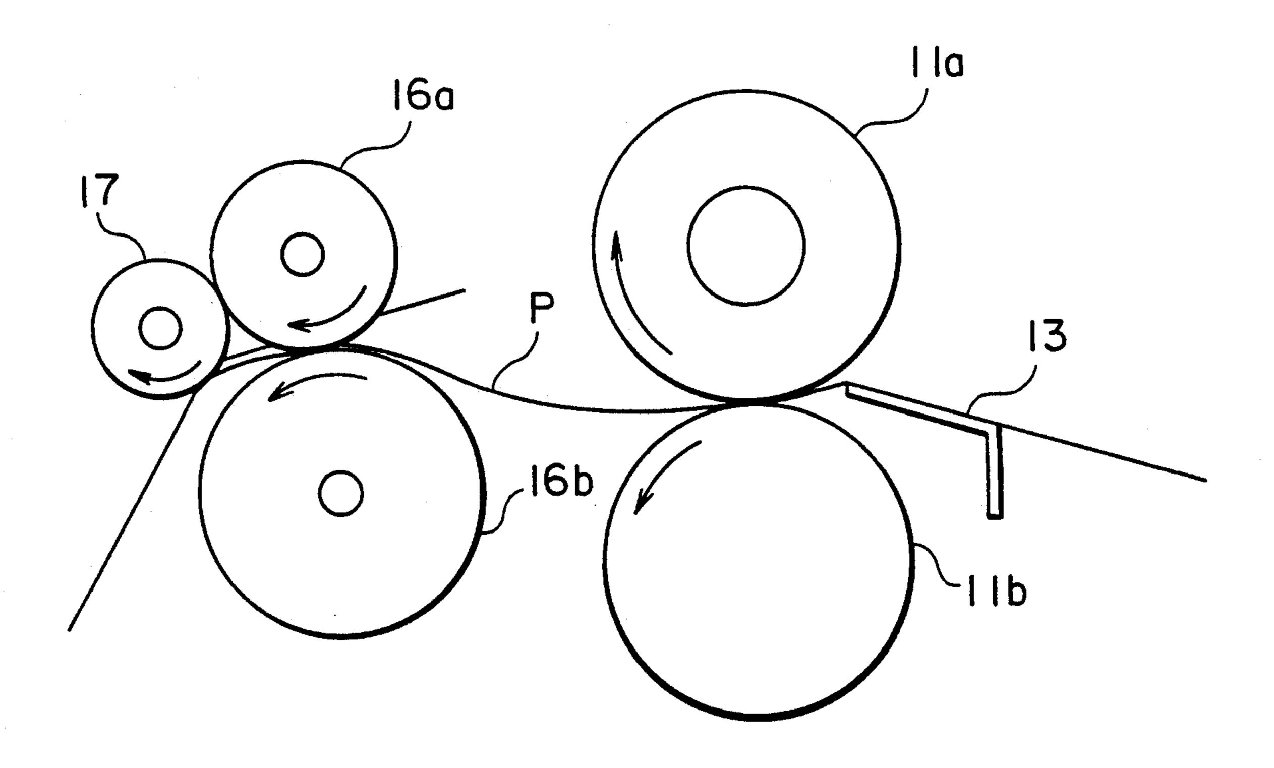
face deviates with buckling from the paper-transport path in the fixing apparatus.
