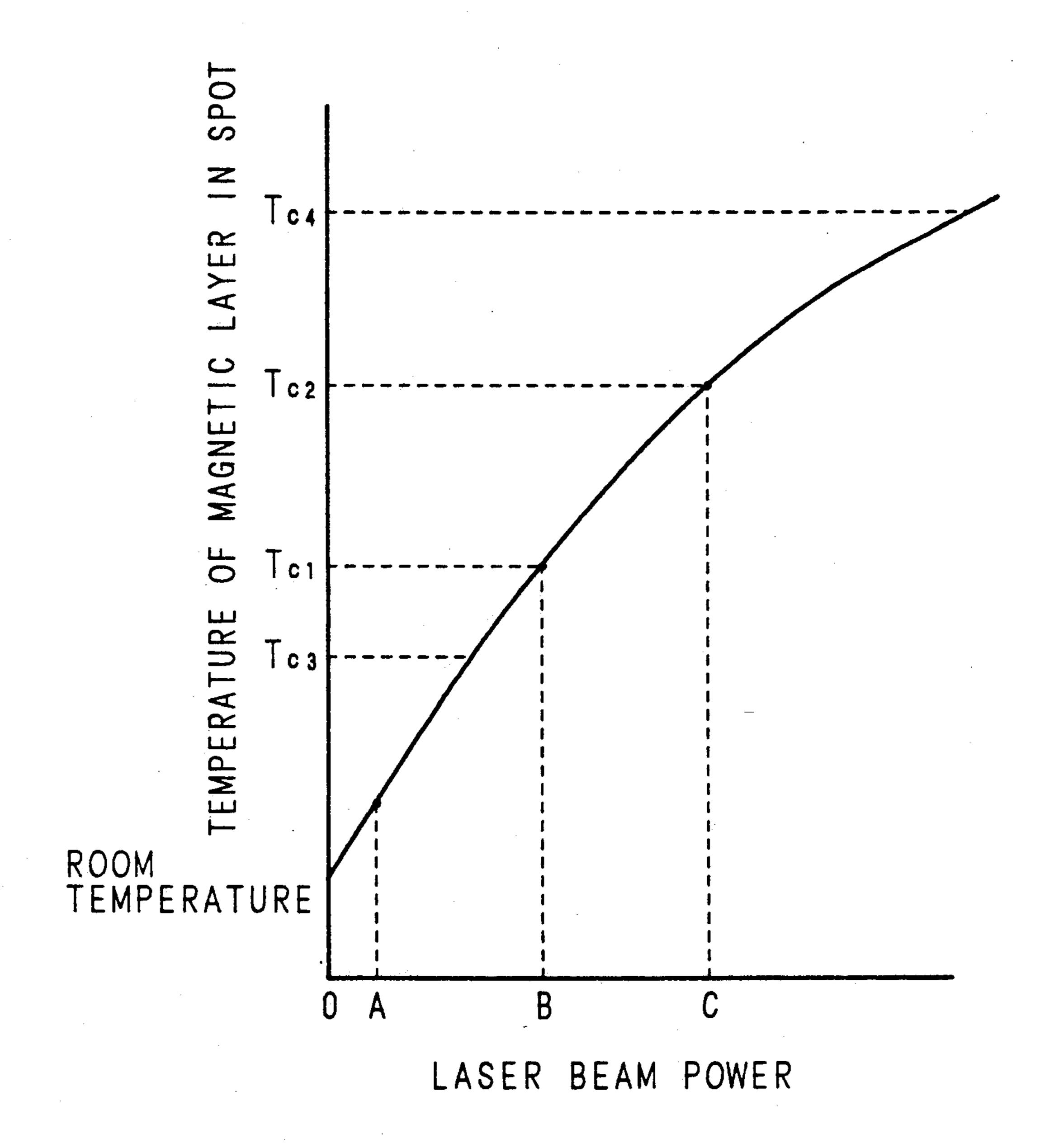
A:POWER IN READING OUT DATA B:POWER IN RECORDING DATA 'O' C:POWER IN RECORDING DATA '1'
