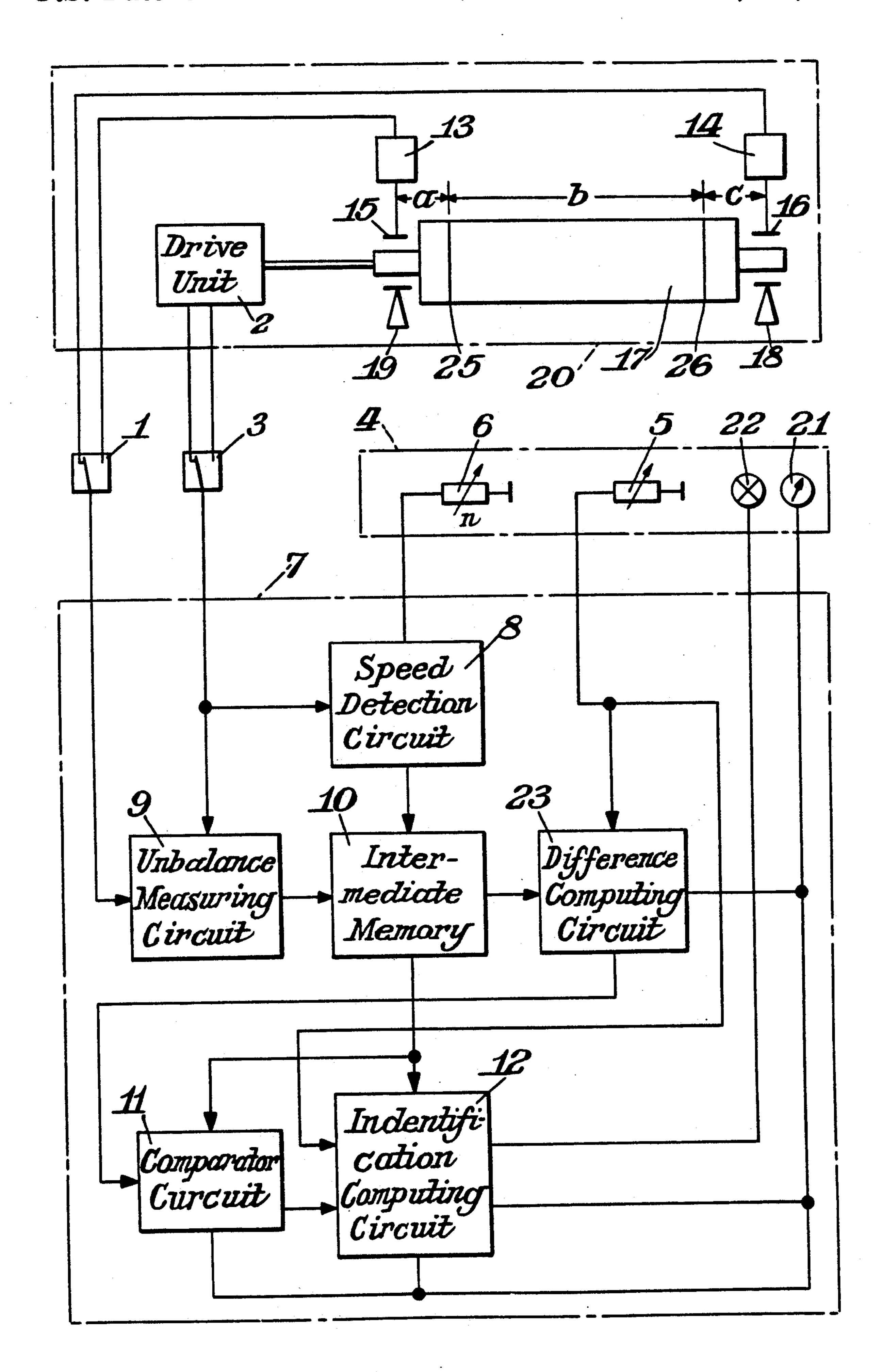
PROCESS AND DEVICE FOR AUTOMATIC IDENTIFICATION OF INCREASED RESONANCE RESPONSE DURING BALANCING PROCEDURE
