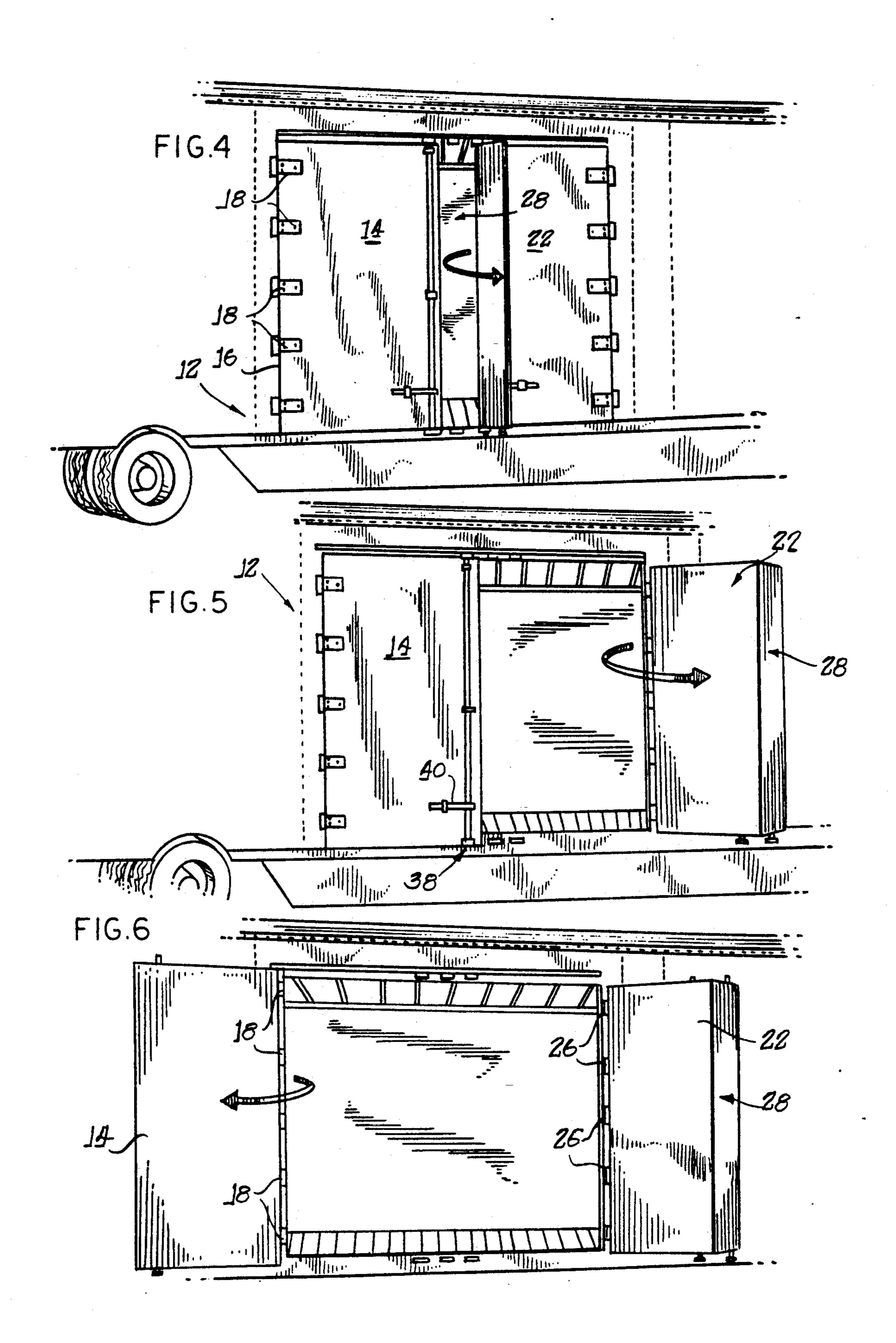
FIG. 5 is a view similar to FIG. 4 showing a progressive, intermediate opening of the door structure; and
