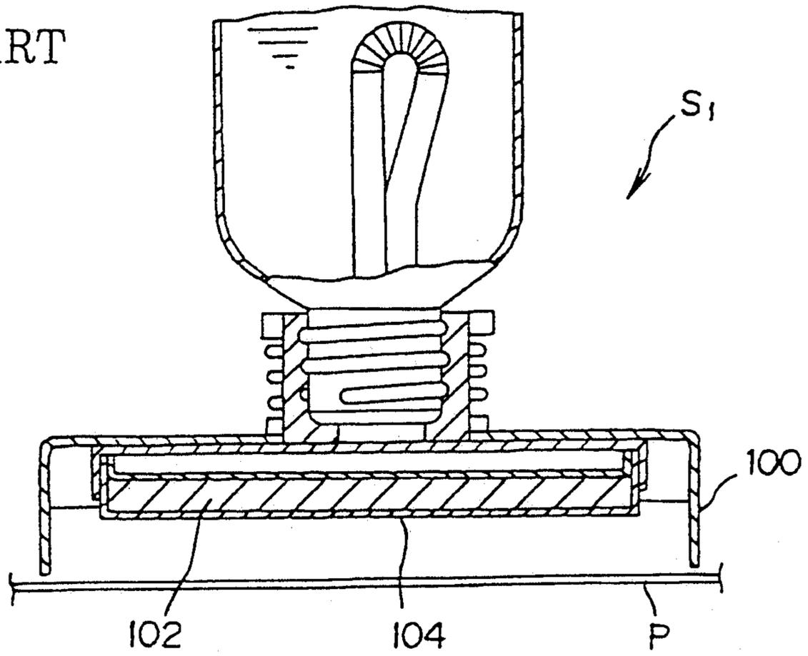
**STAMP DEVICE EMPLOYING A HEAT SENSITIVE STENCIL PAPER TO BE PERFORATED BY HEAT OF A THERMAL HEAD**
