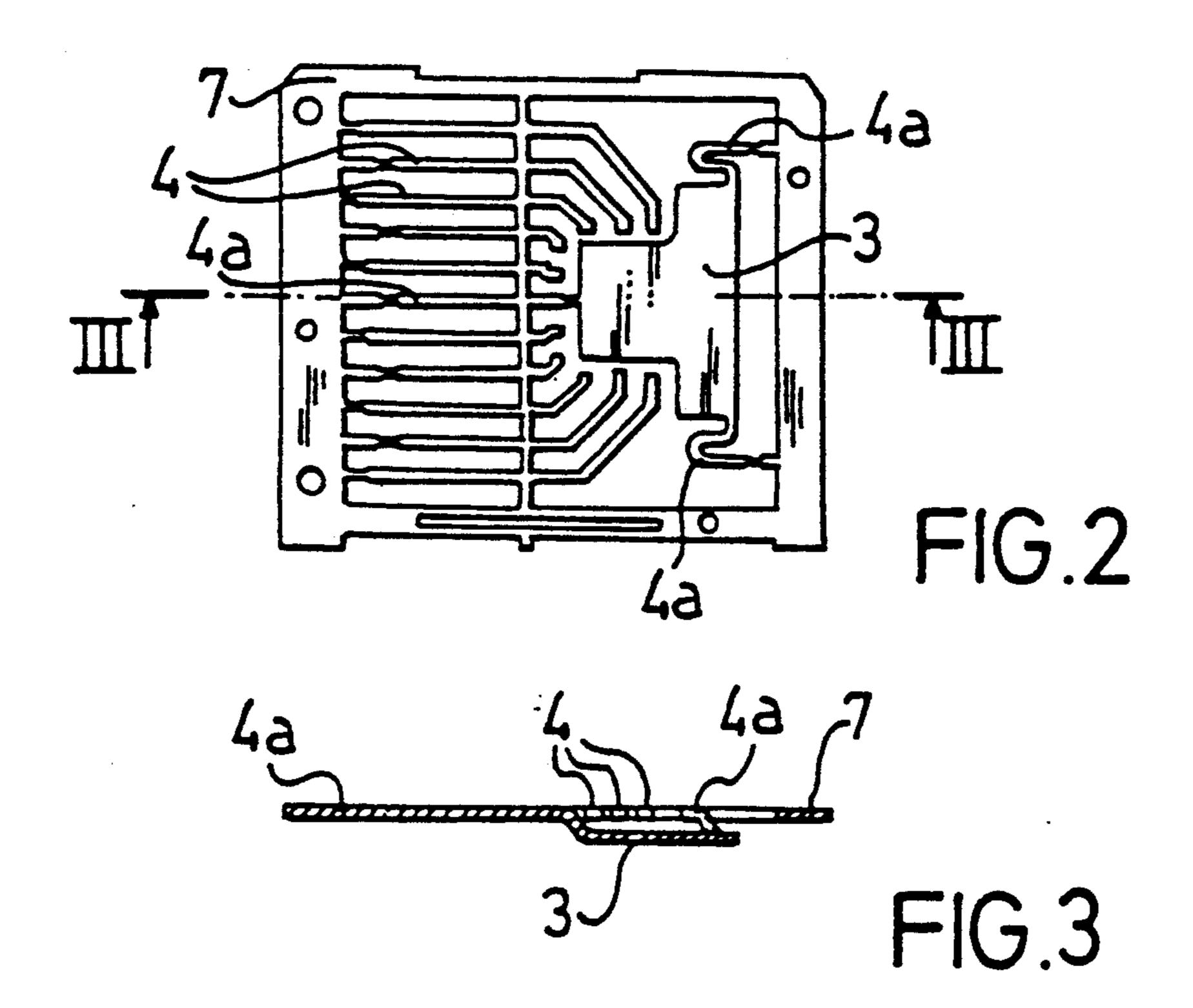
MOLD FOR MANUFACTURING PLASTIC INTEGRATED CIRCUITS INCORPORATING A HEAT SINK
