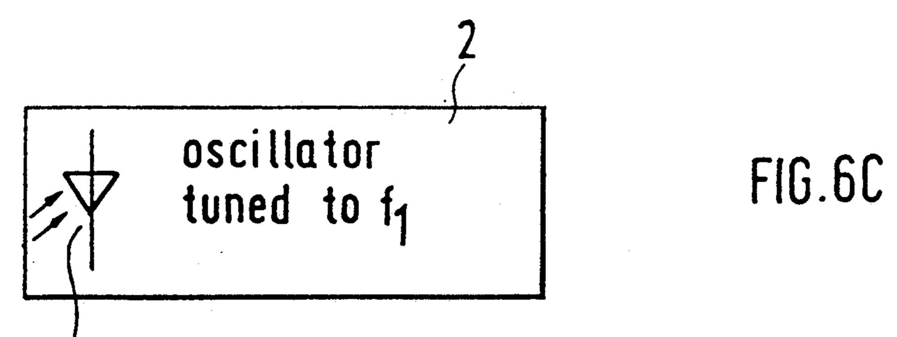
photosensitive transit-time device (photo-Baritt-diode or photo-Gunn-diode or photo - Impatt-diode)
