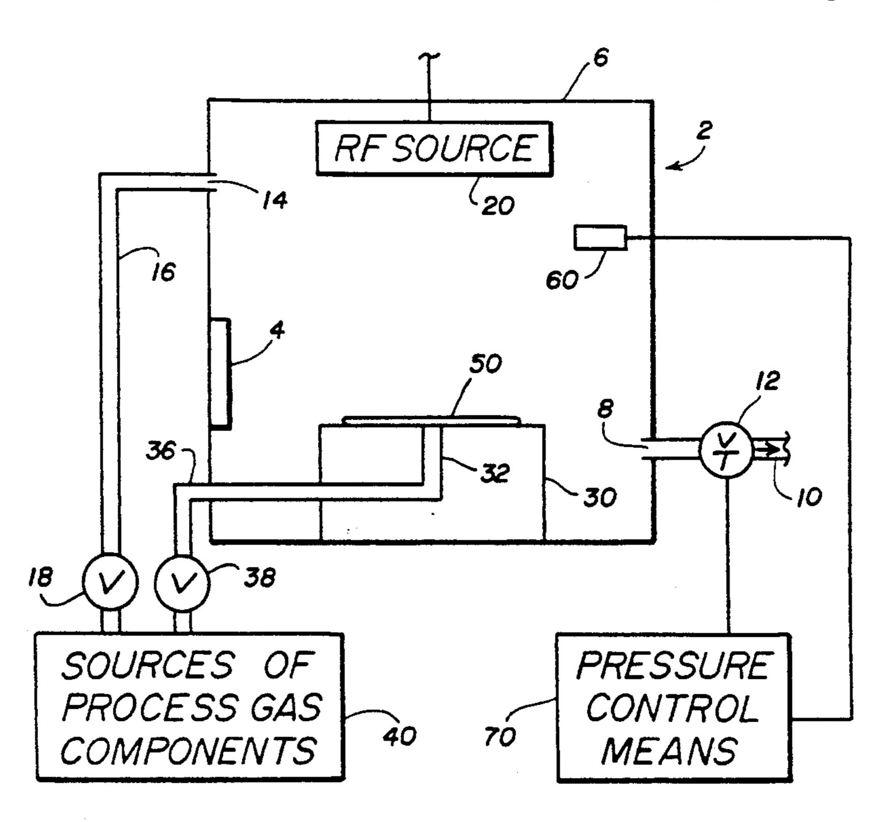
NONSEALINGLY SUPPORTING A SEMICONDUCTOR WAFER ON A HEATSINK IN A PLASMA ETCHING CHAMBER
