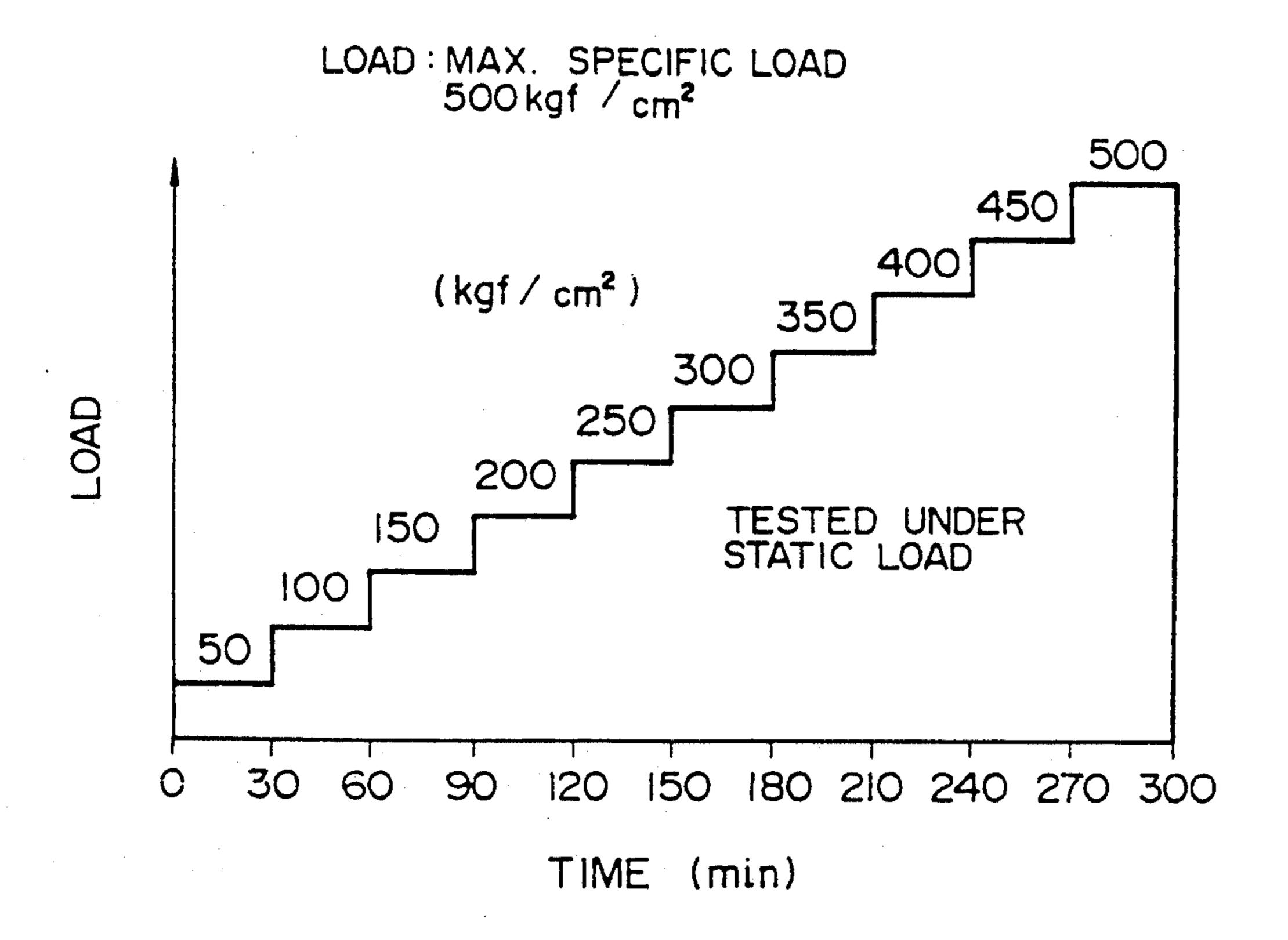
EVALUATION METHOD: SEIZURE IS JUDGED WHEN BEARING BACK TEMPERATURE RISES OVER 200°C, OR FRICTION RESISTANCE RISES OVER 50 kgf·cm
