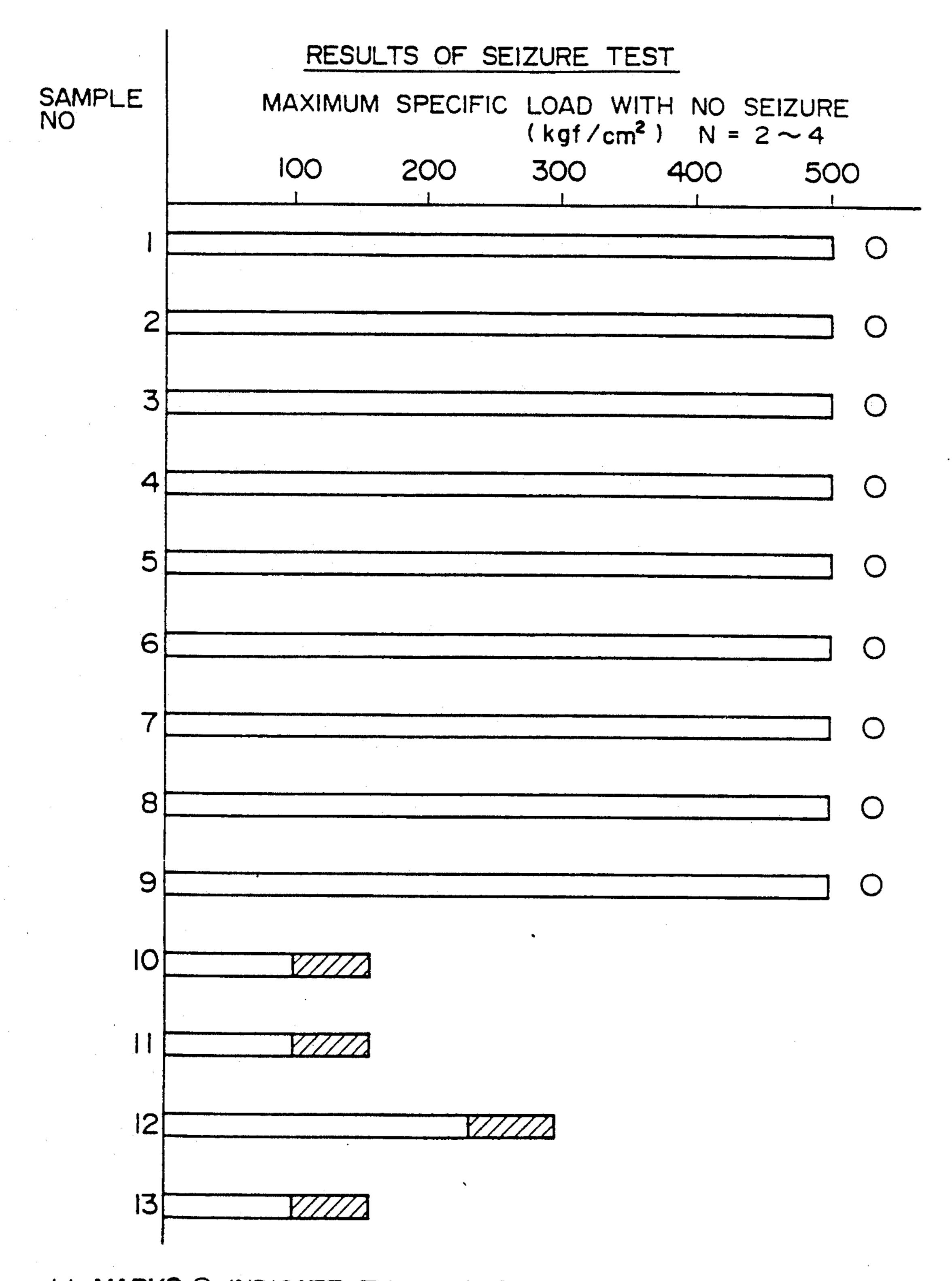
\*1: MARKS O INDICATE THAT NO SEIZURE WAS OBSERVER MARKS ZZINDICATE VARYING RANGES OF TEST RESULTS
