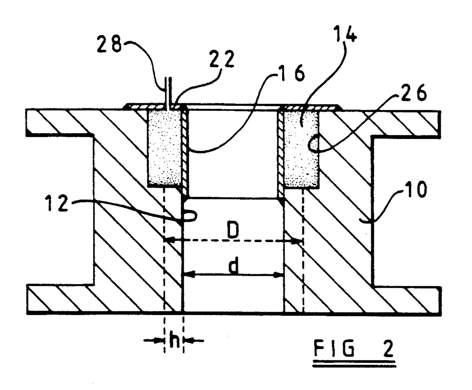
This invention relates to a gear, and is more particularly concerned with an internal gear for use in applica- 5 tions where corrosion of the gear teeth present a problem. Such a problem is encountered with gears used in rotary actuators, particularly aircraft actuators, and more particularly actuators of the geared hinge type which are used for operating the leading edge flying 10 control surfaces on certain types of aircraft
