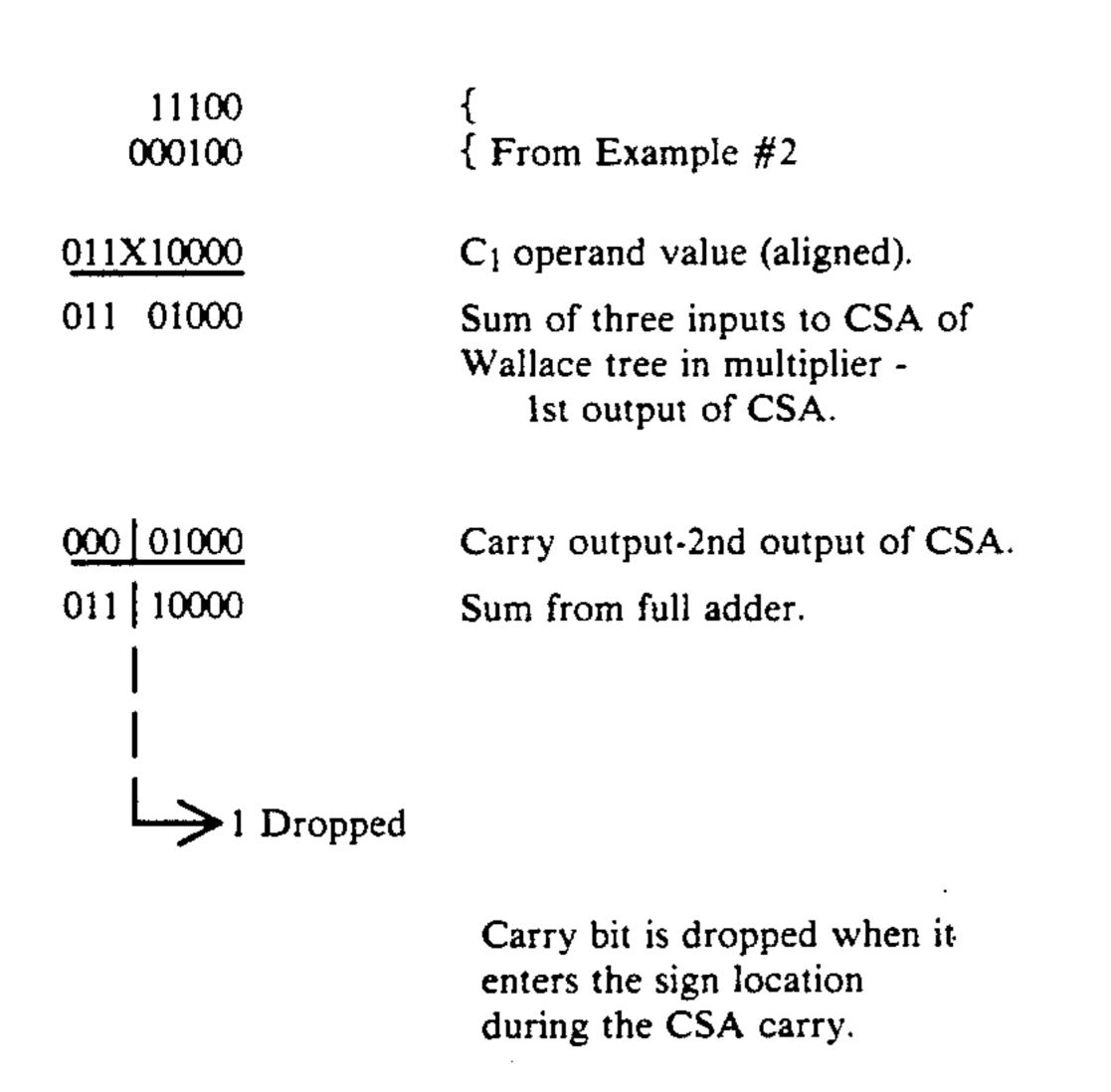
A similar situation exists for the example identified as #3. In this case a C<sub>2</sub> operand value is added. Again, the 60 carry bit is dropped when it enters the sign location, but now this occurs during addition preceding the full add cycle.
