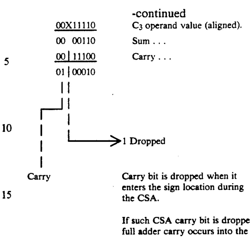
If such CSA carry bit is dropped, and a full adder carry occurs into the sign position, the full adder carry is propagated to the next MSB.
