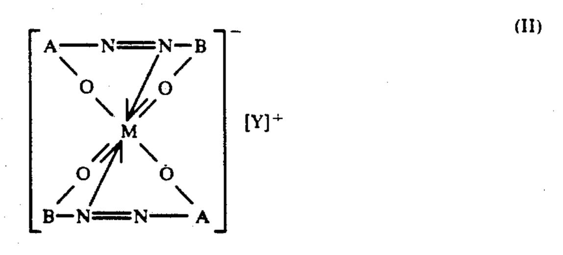
(wherein A is a residual group of a diazo component having a phenolic hydroxyl group at the ortho-position; B is a residual group of a coupling component; M is a chromium, iron, aluminium, zinc or cobalt atom; and [Y]+ is an inorganic or organic cation).
