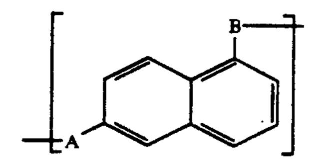
wherein A and B, which can be either equal to, or different, from, each other, can be either —O— or — CO— and one of the following moieties:
