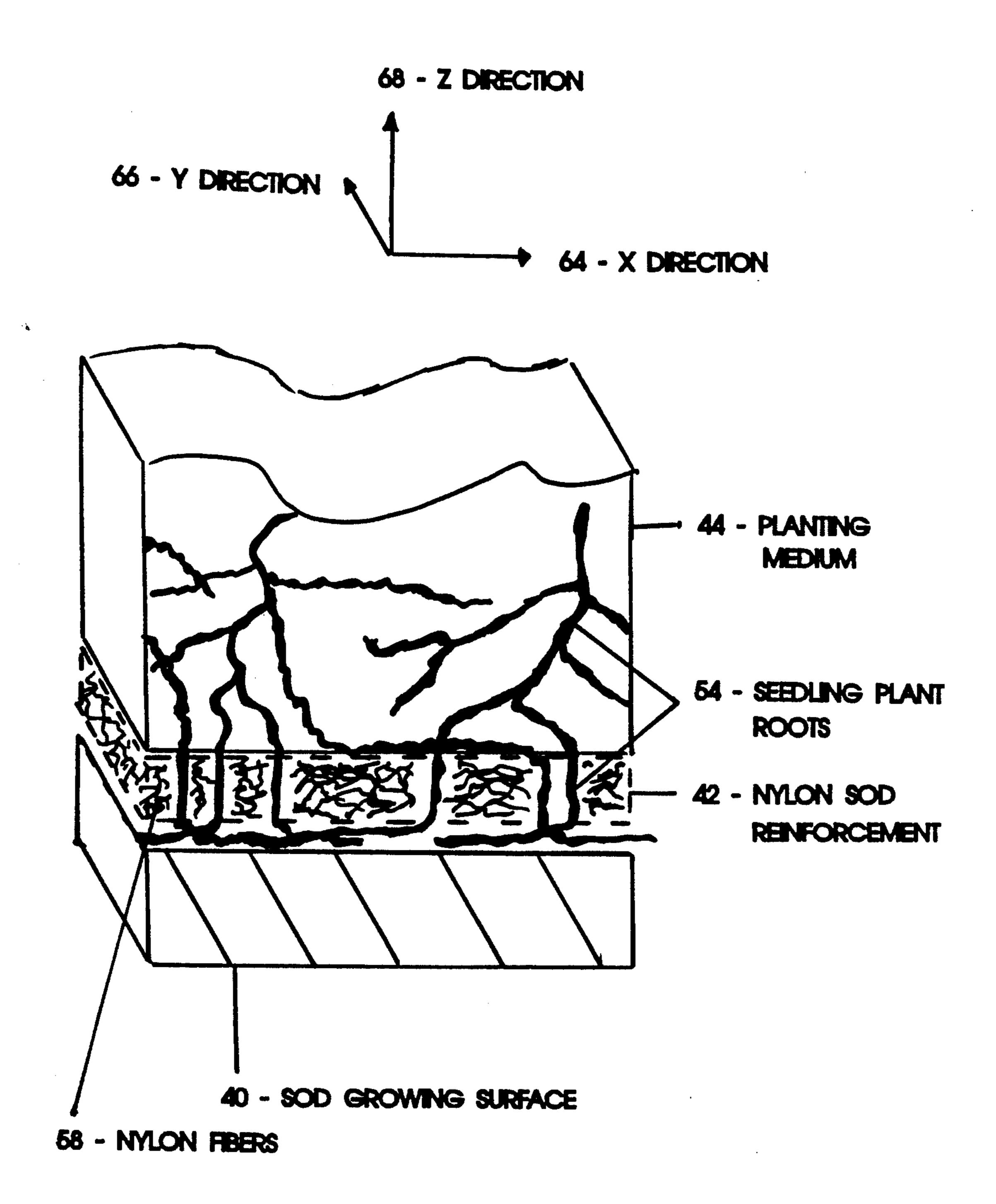
**FIG.** 3 EXPLODED VIEW OF ROOT PENETRATION IN AREA BONDED NYLON SPUNBOND FABRIC
