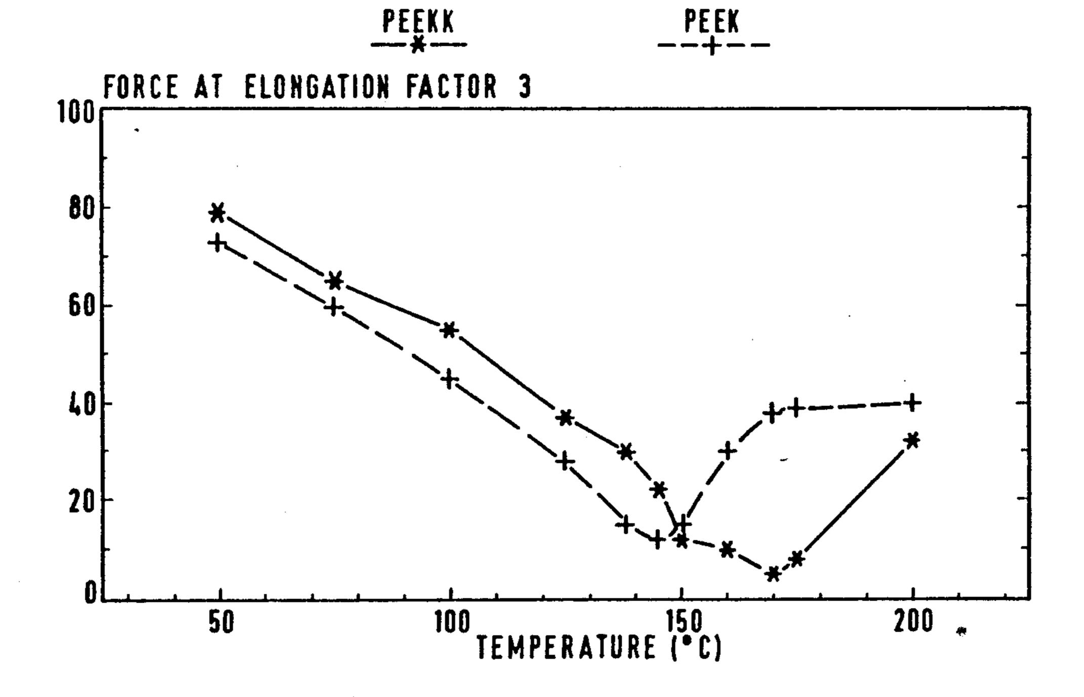
PEEKK-AND PEEK TENSIL FORCE MORPHOUS BETWEEN TEMPERATURE A HEATED CHAMBER RMOPLASTIC BEHAVIOUR OF PEEKK ELONGATION ELONGATION IN ATIONSHIP
