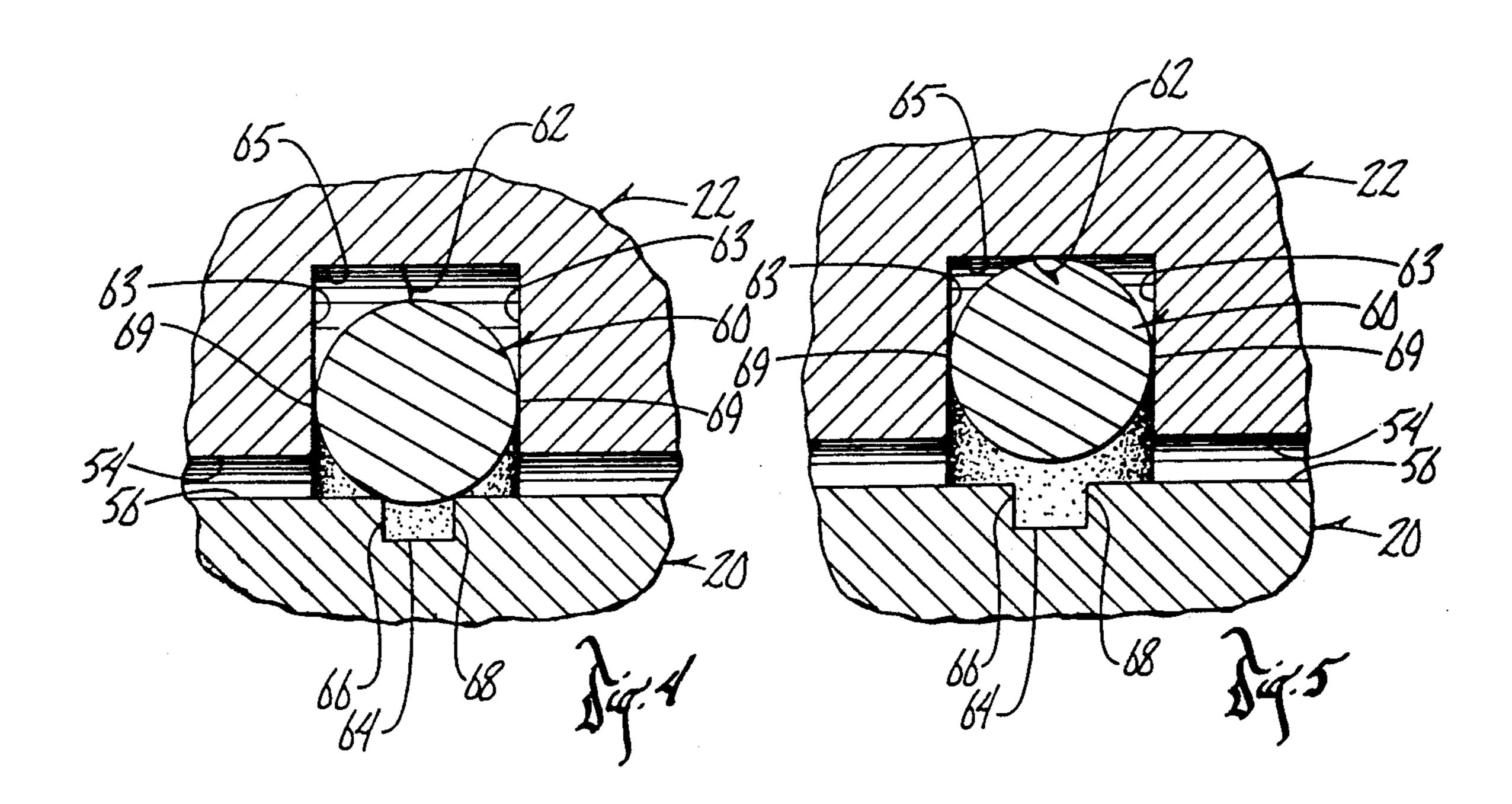
STATIC AND DYNAMIC SHAFT SEAL ASSEMBLY
