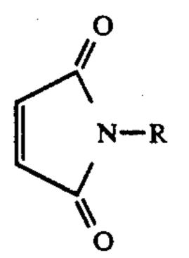
where R is C<sub>3</sub>-C<sub>30</sub> alkyl radical comprising and 5-amino-triazole is provided. A lubricating oil composition containing the additive is also provided.
