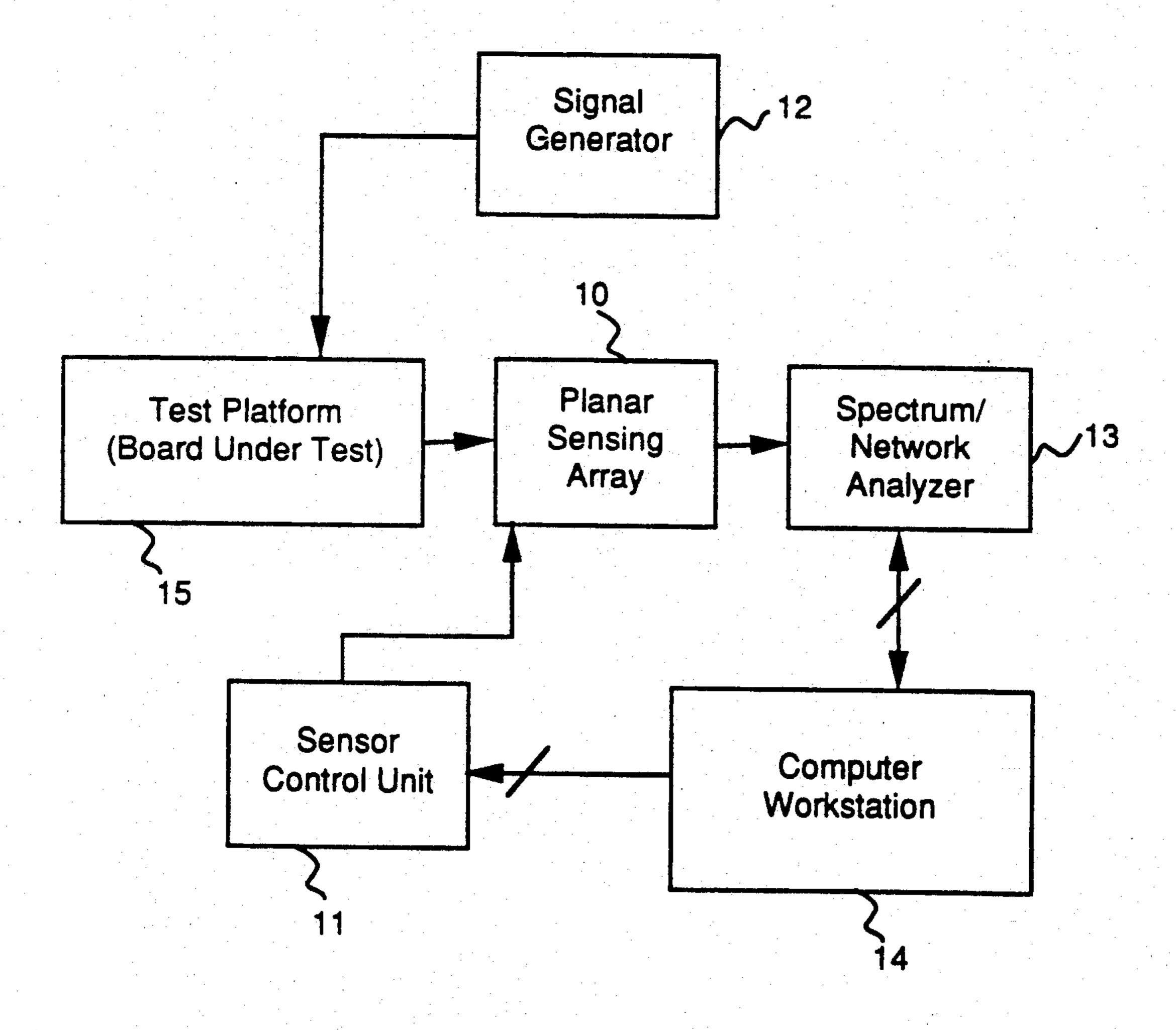
FIG. 1 The Hardware Architecture of the CTS
