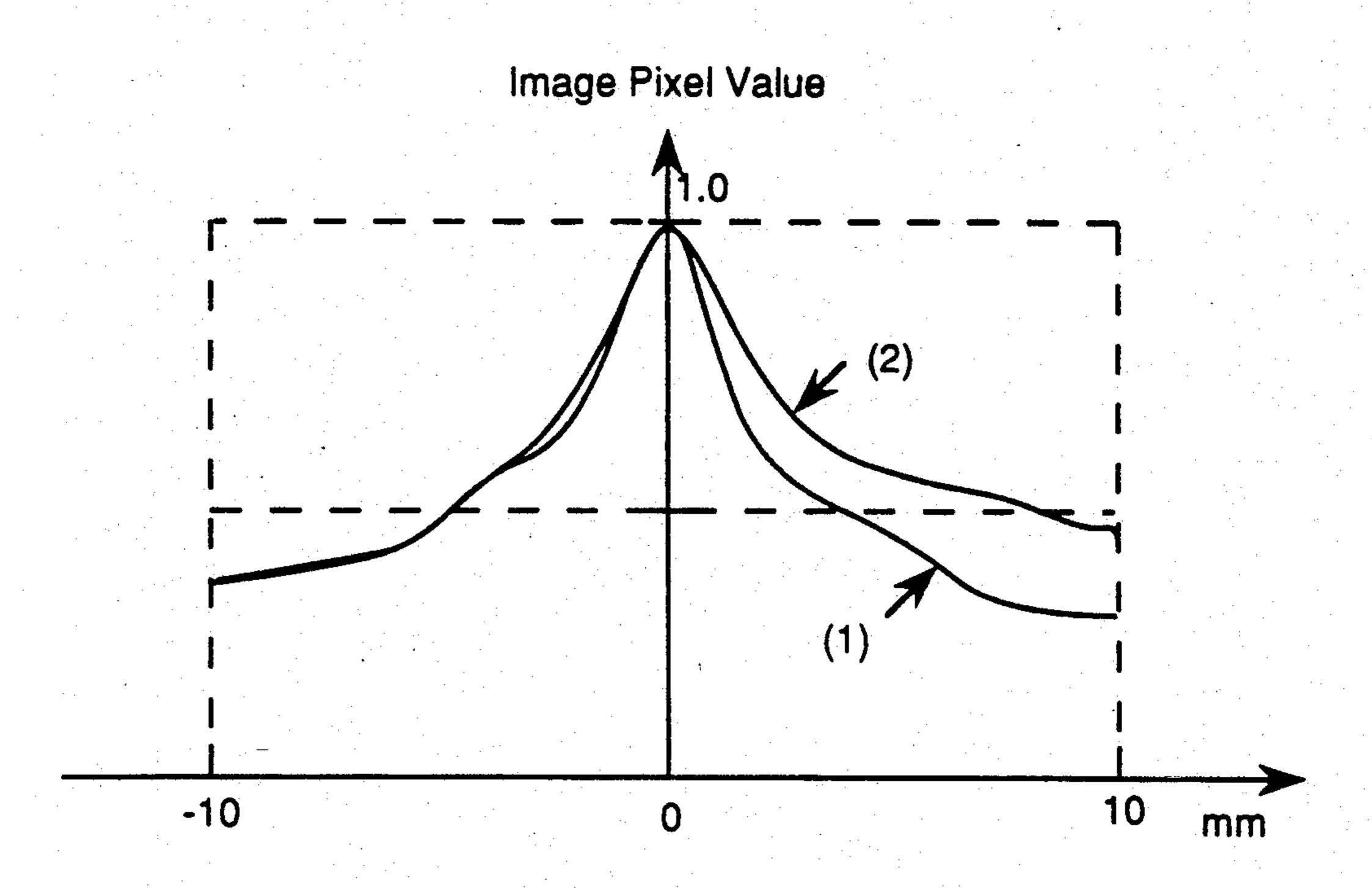
FIG. 4 One Dimensional Images of a Faulty and a Non-faulty boards
