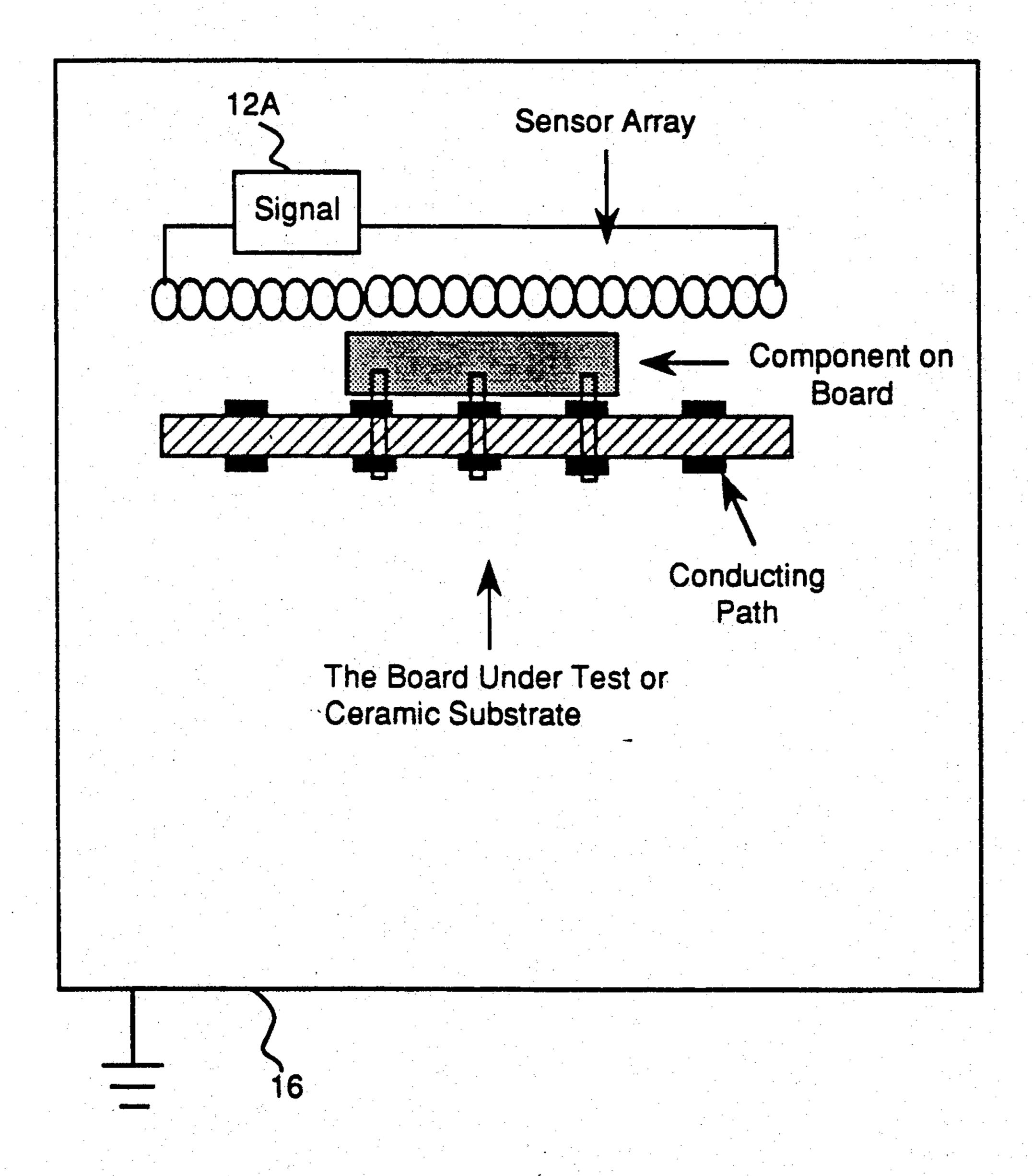
FIG. 3 One Dimensional Sensing Array.
