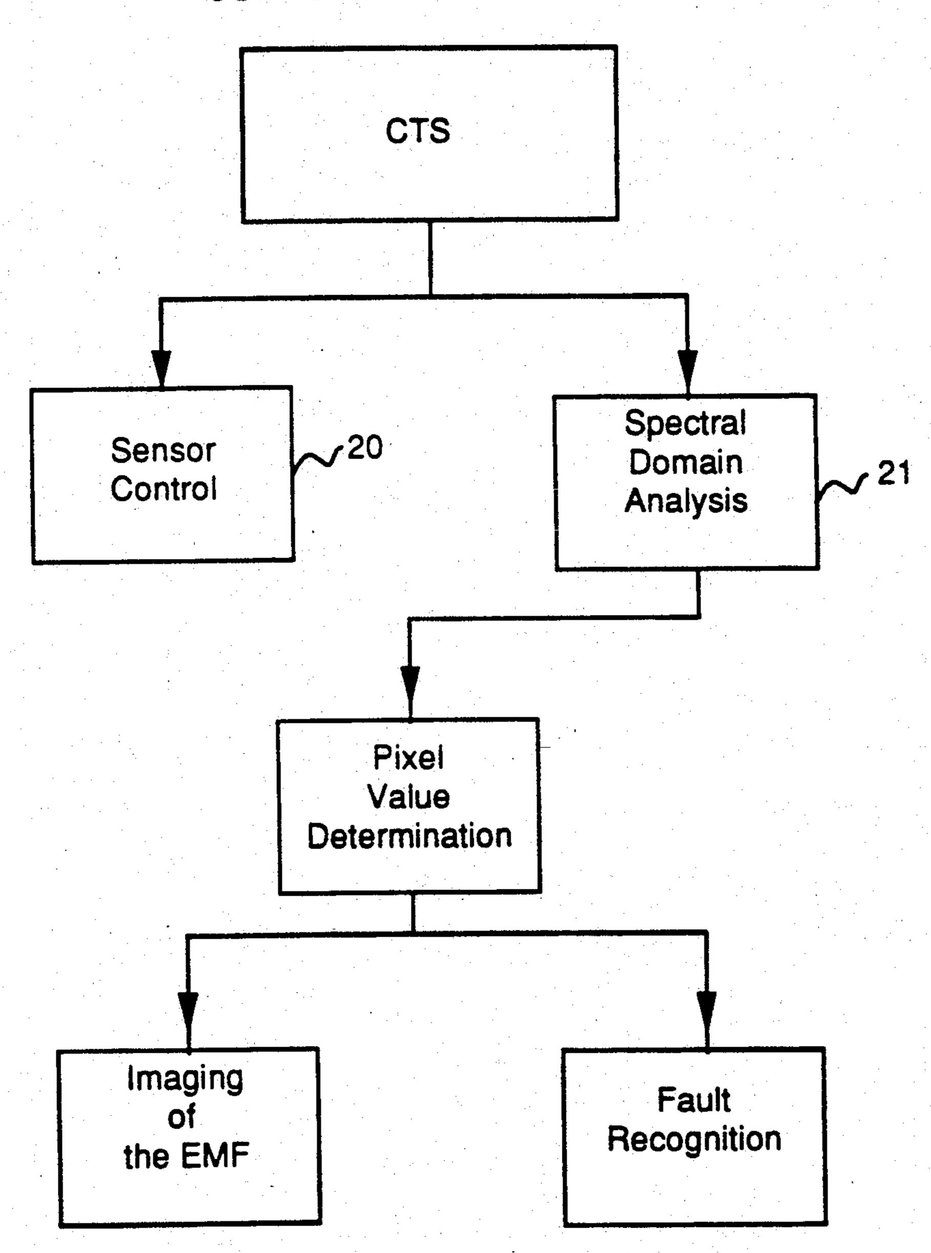
FIG 2. The Software Architecture of the CTS.
