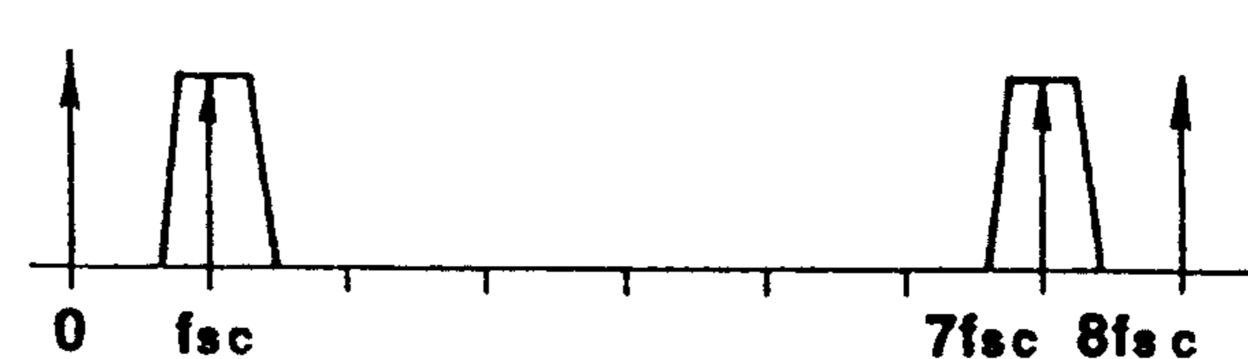
FIG. 3 (G) MODULATED COLOR DIFFERENCE SIGNAL (MOD.C)
