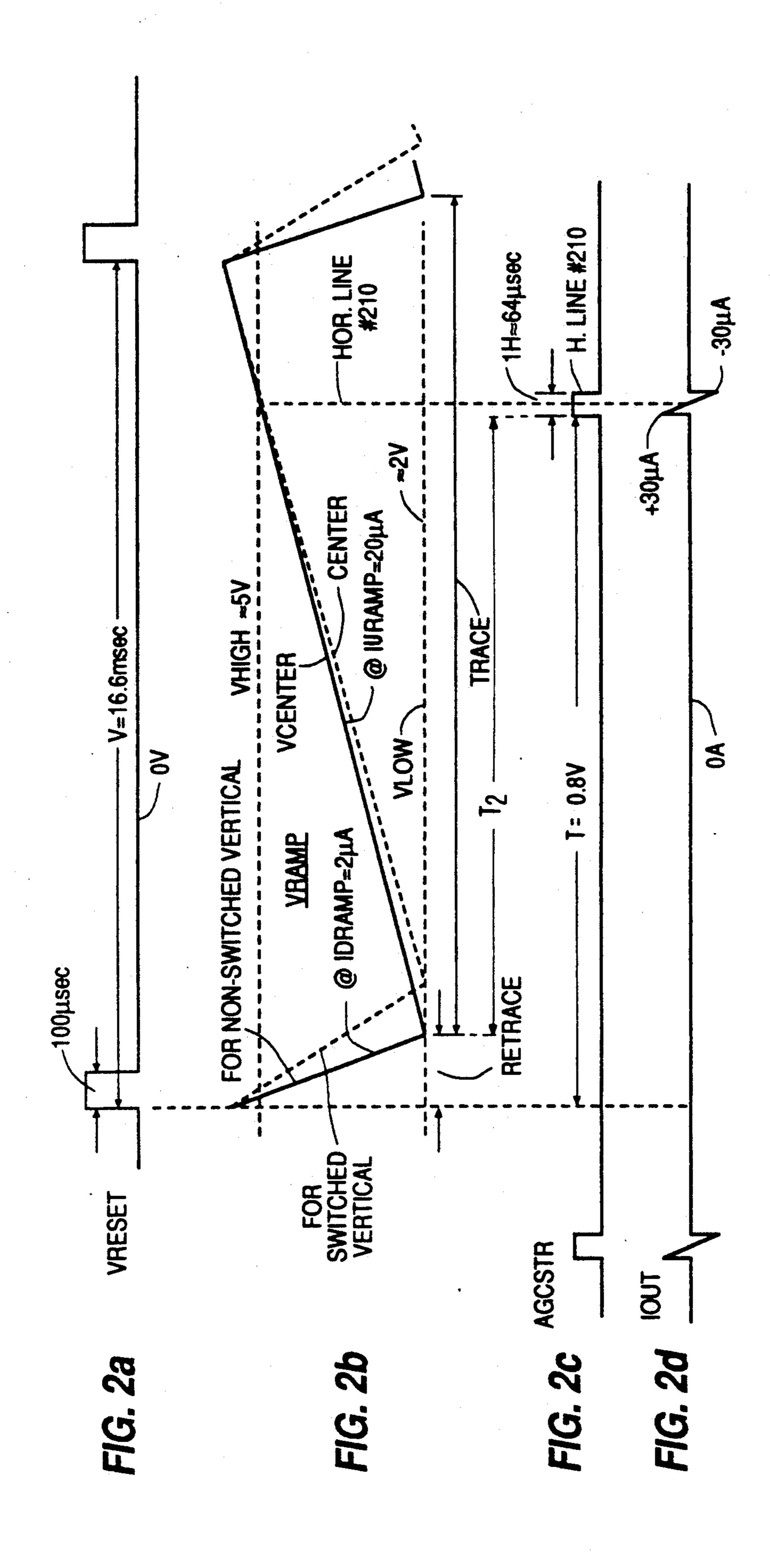
GENERATOR FOR SAWTOOTH SIGNAL WITH SELECTABLE RETRACE SLOPE FOR A DEFLECTION APPARATUS
