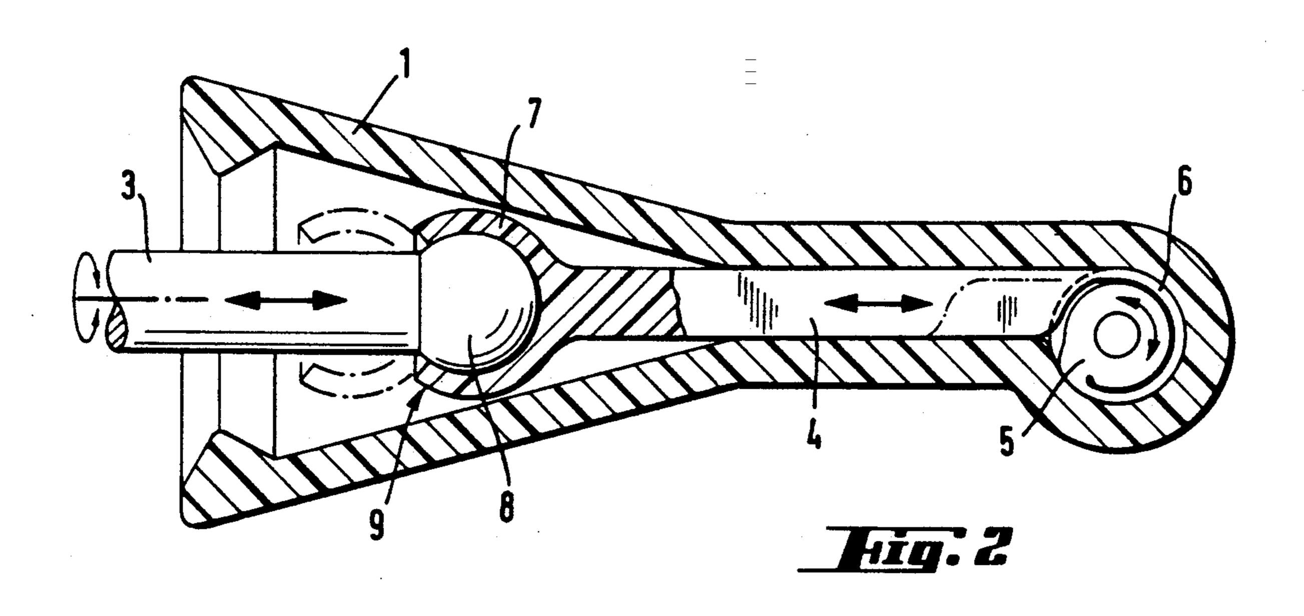
WORK DEVICE SHAFT FOR THE ELECTRIC DRIVE MECHANISM OF A TOOTHBRUSH
