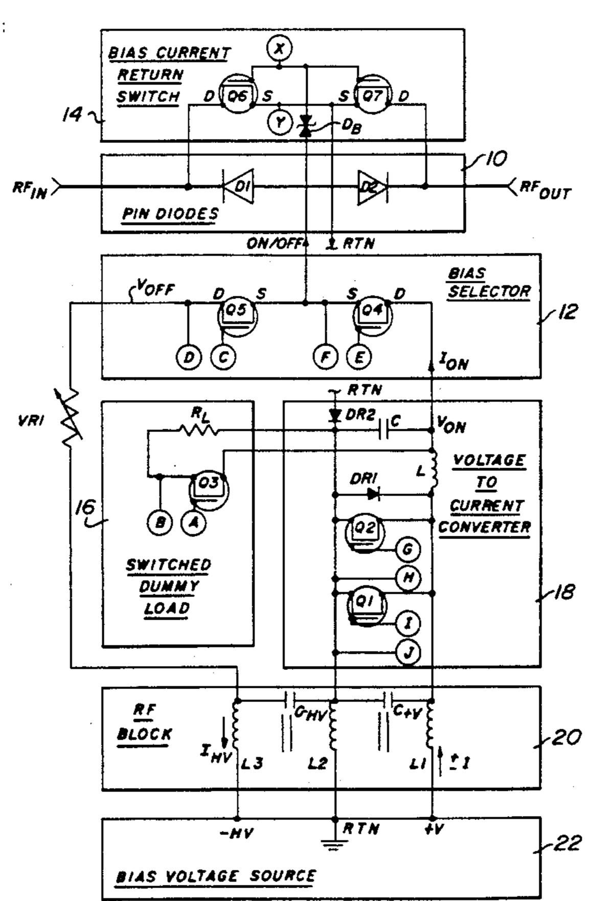
"Broadbanding the Shunt PIN-diode SPDT Switch",
