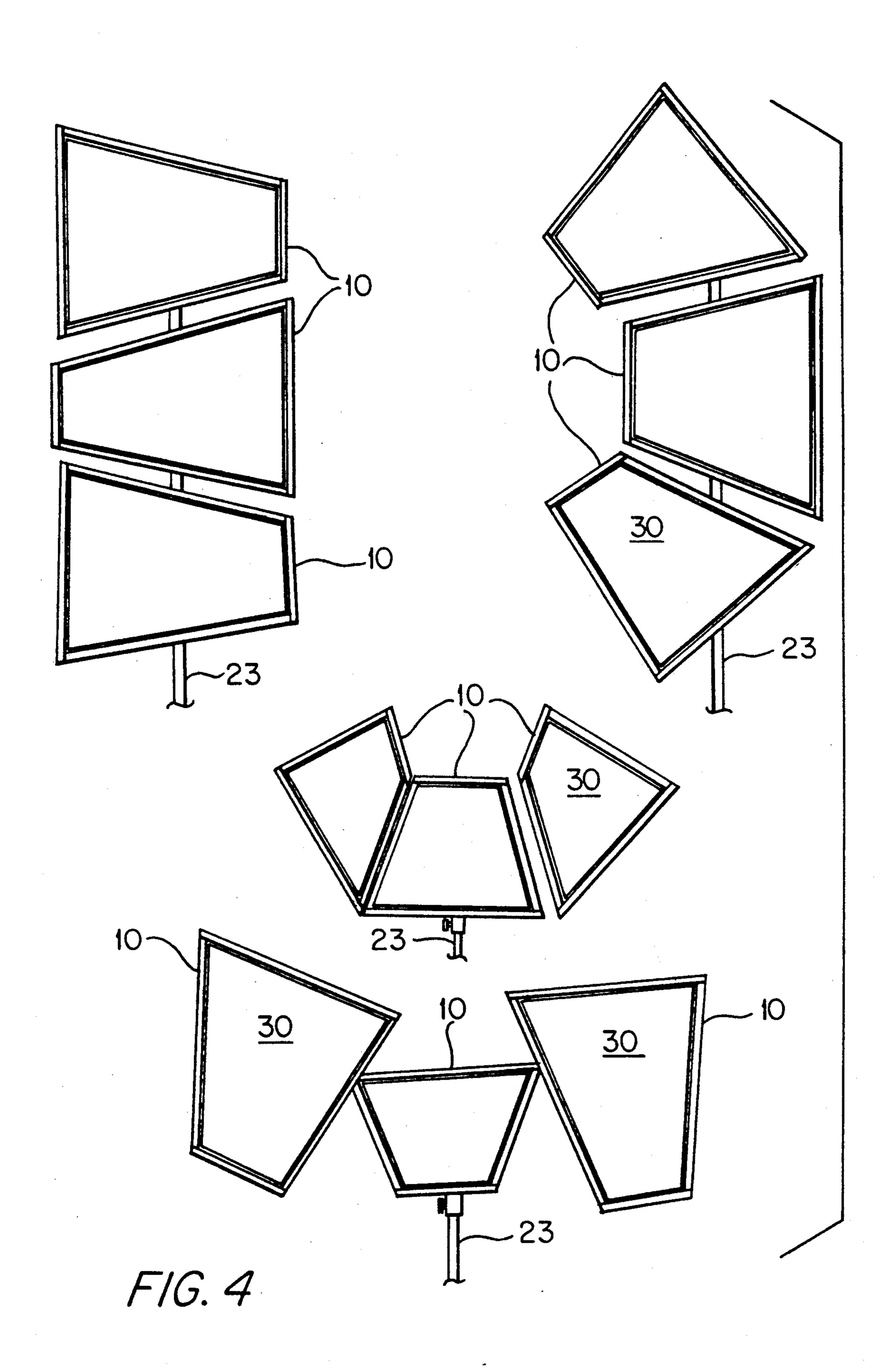
The light-reflecting frames may carry light-reflecting surfaces which are detachably attached to the frames e.g. by elasticated cord.
