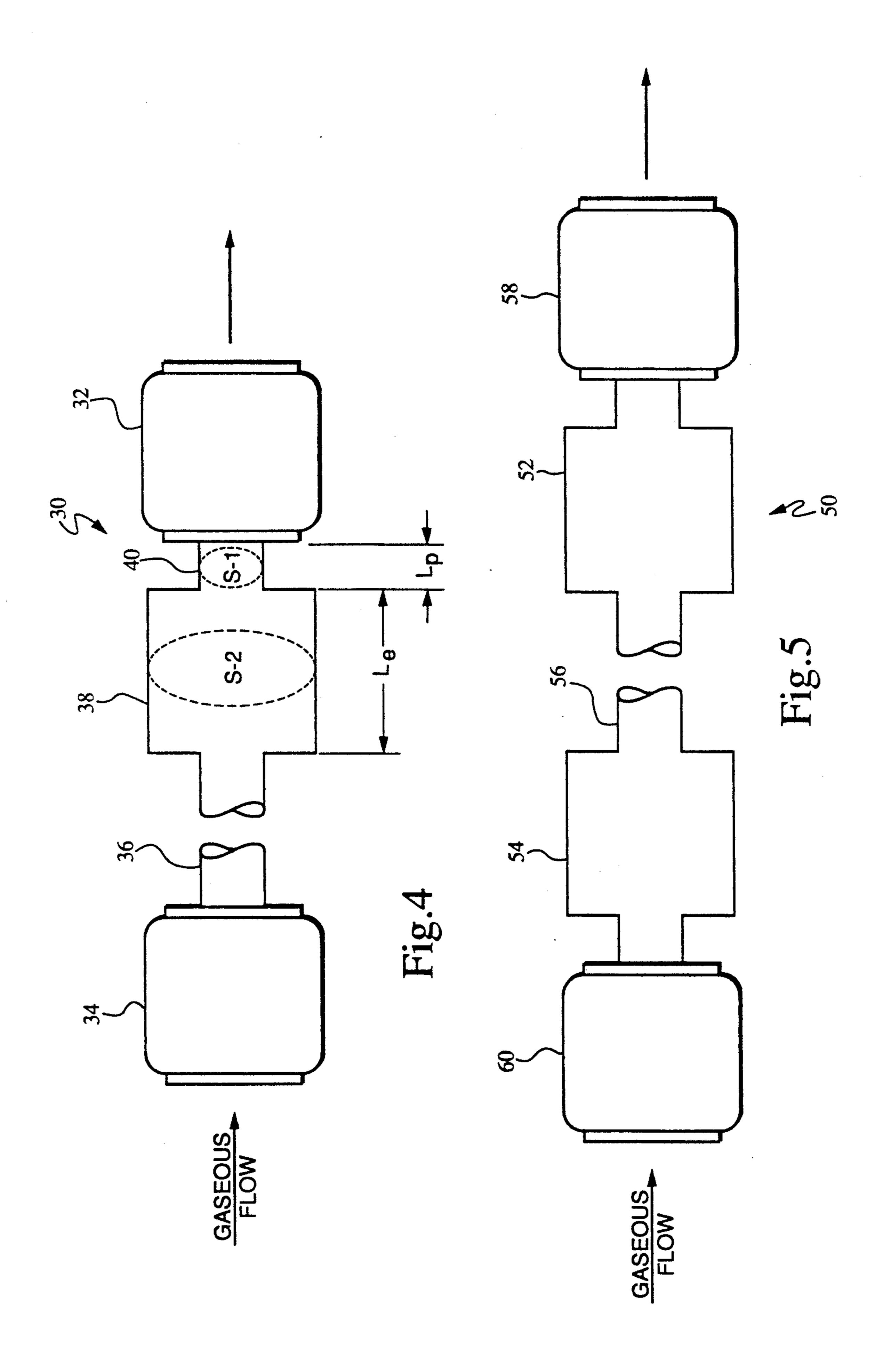
to a hose, tubing, or pipe 12 with the inlet to the tubing open to free space, the tube becomes a tuned one-quarter wavelength cavity. Such a cavity will resonate with sound waves at a fundamental frequency with a wavelength of four times the length of the cavity:
