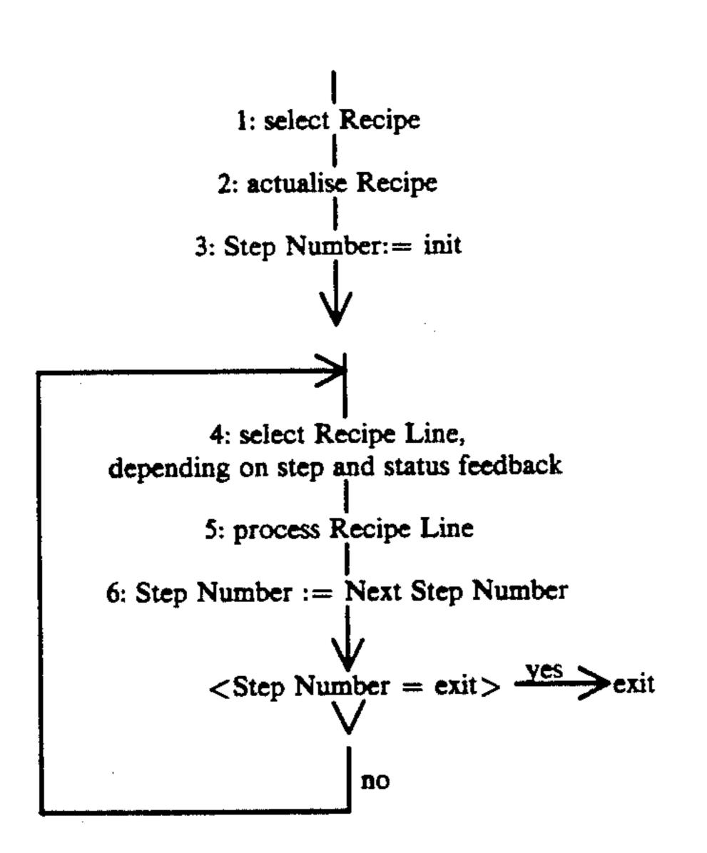
1. The work station controller selects a Recipe that has an identifier that matches the Operation Description of an
