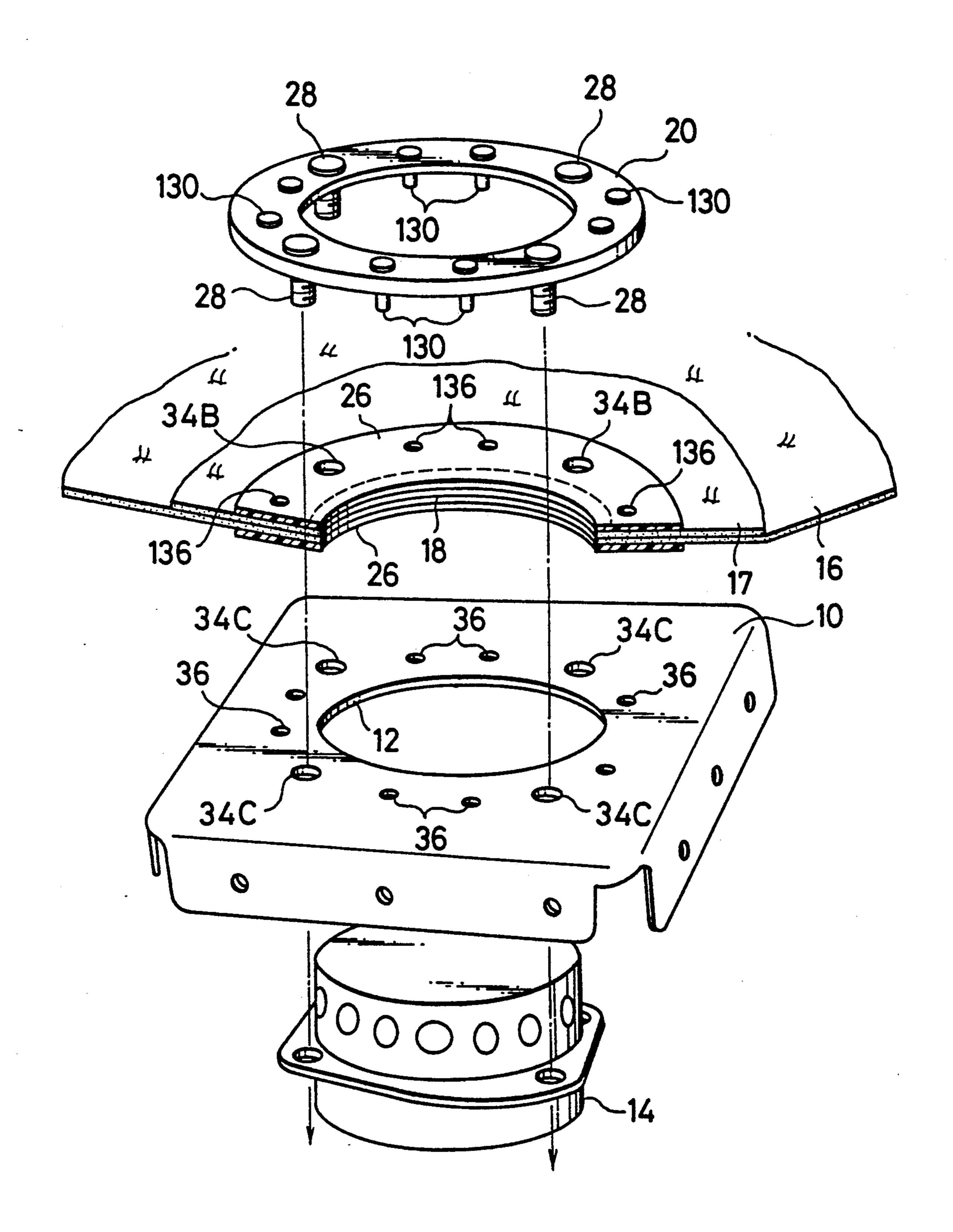
an air bag is reinforced so that its attaching strength is high.
