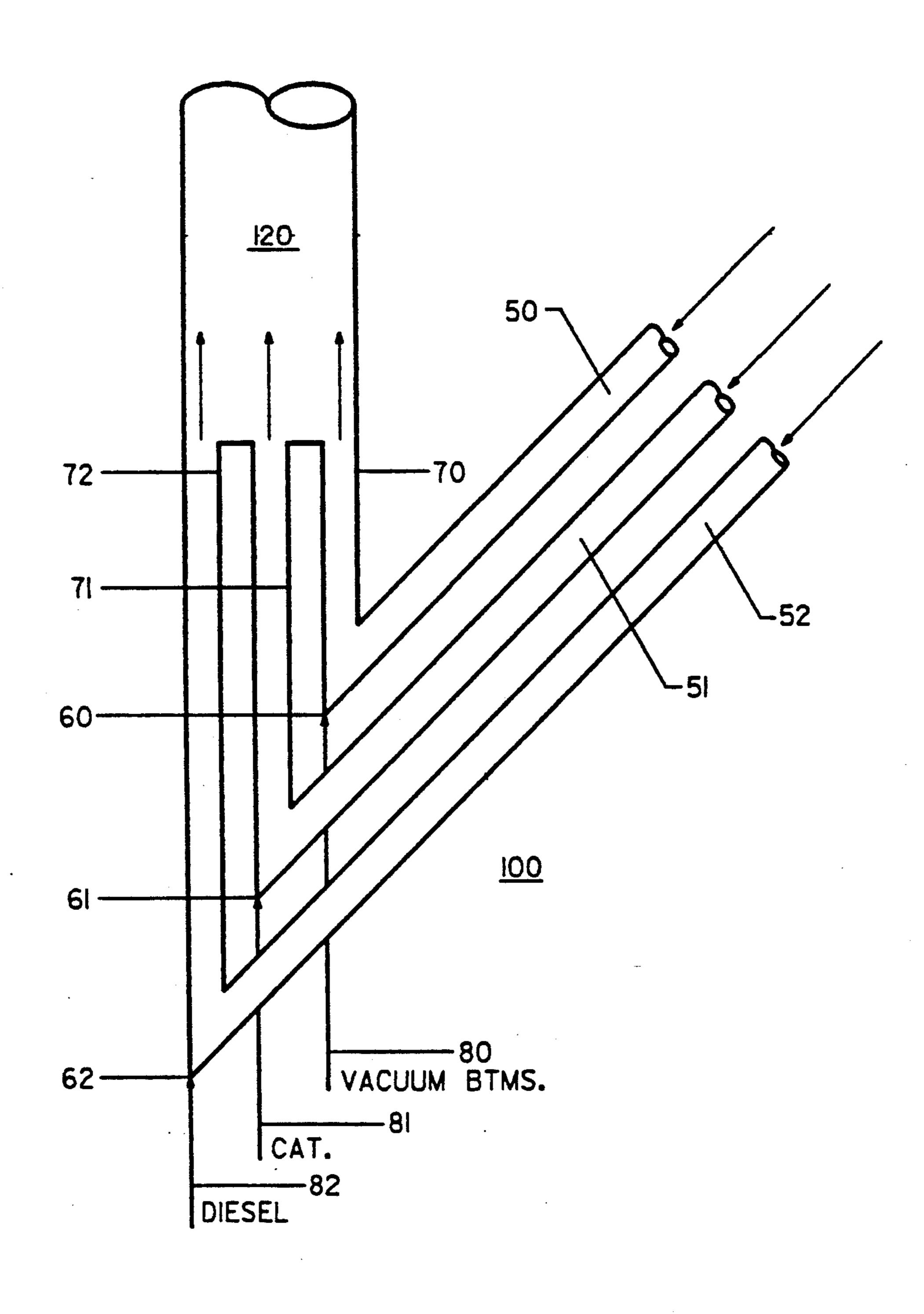
MULTIPLE WYE CATALYTIC CRACKER AND PROCESS FOR USE
