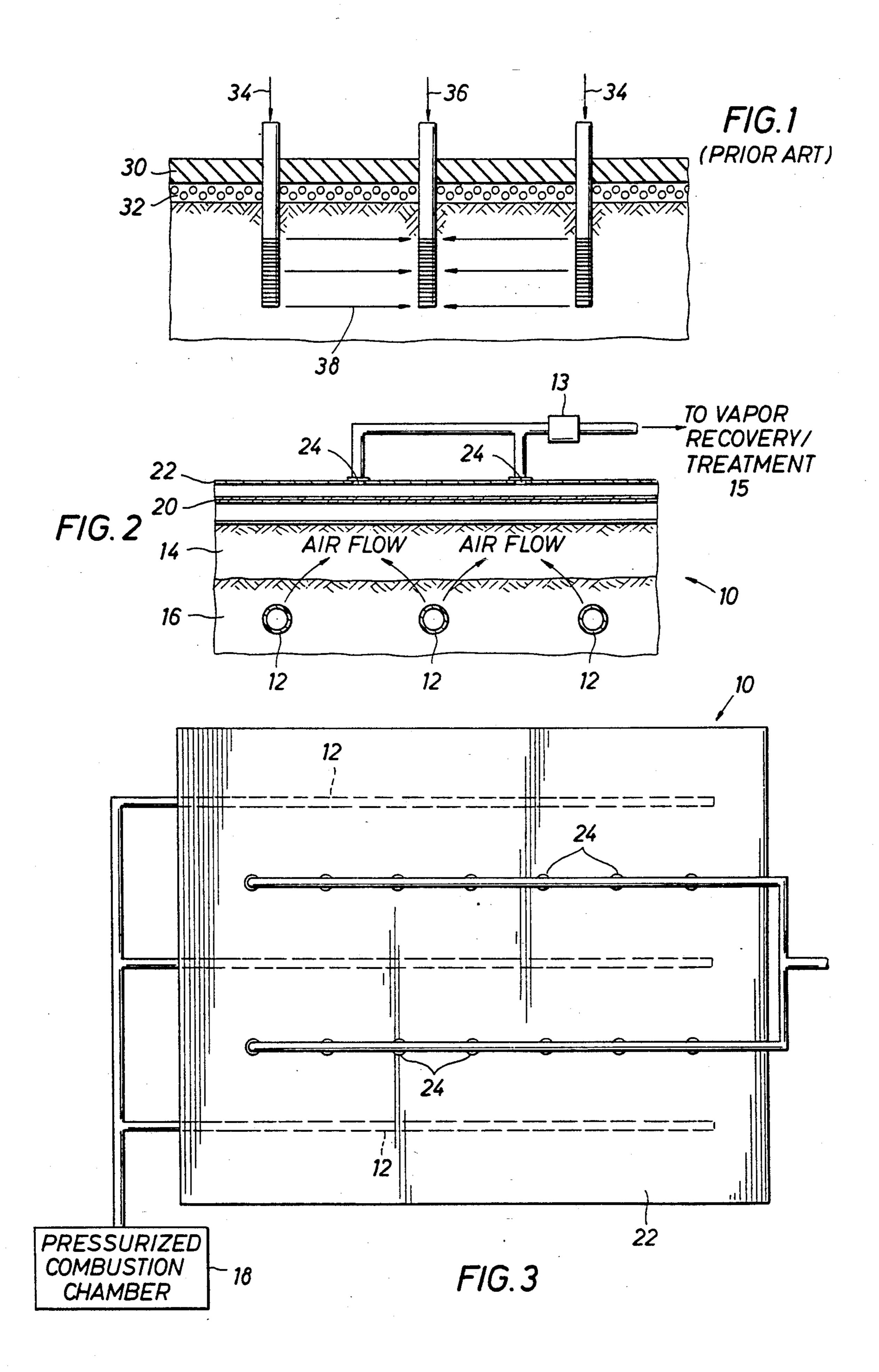
moving from heated soil the vapors formed when soil contaminated by organic contaminants is heated.
