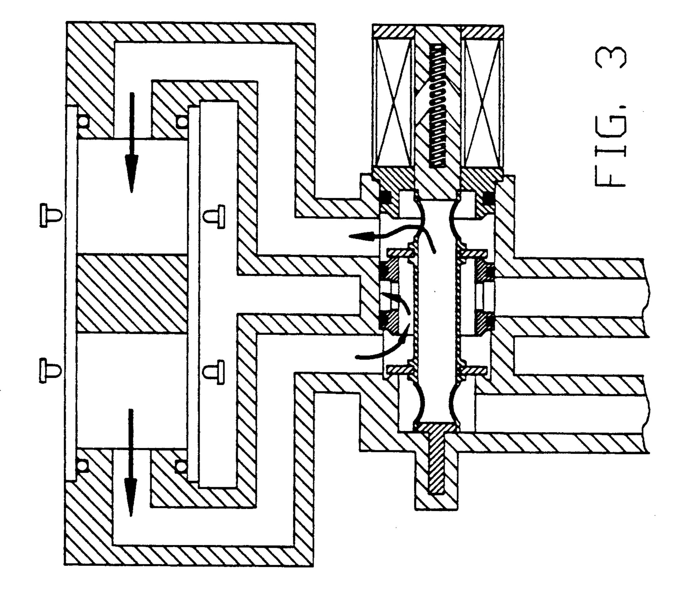
valve body, and for aligning said outlet port with the opening in said sliding valve member at its opposite end, when said sliding valve member is adjacent said first
