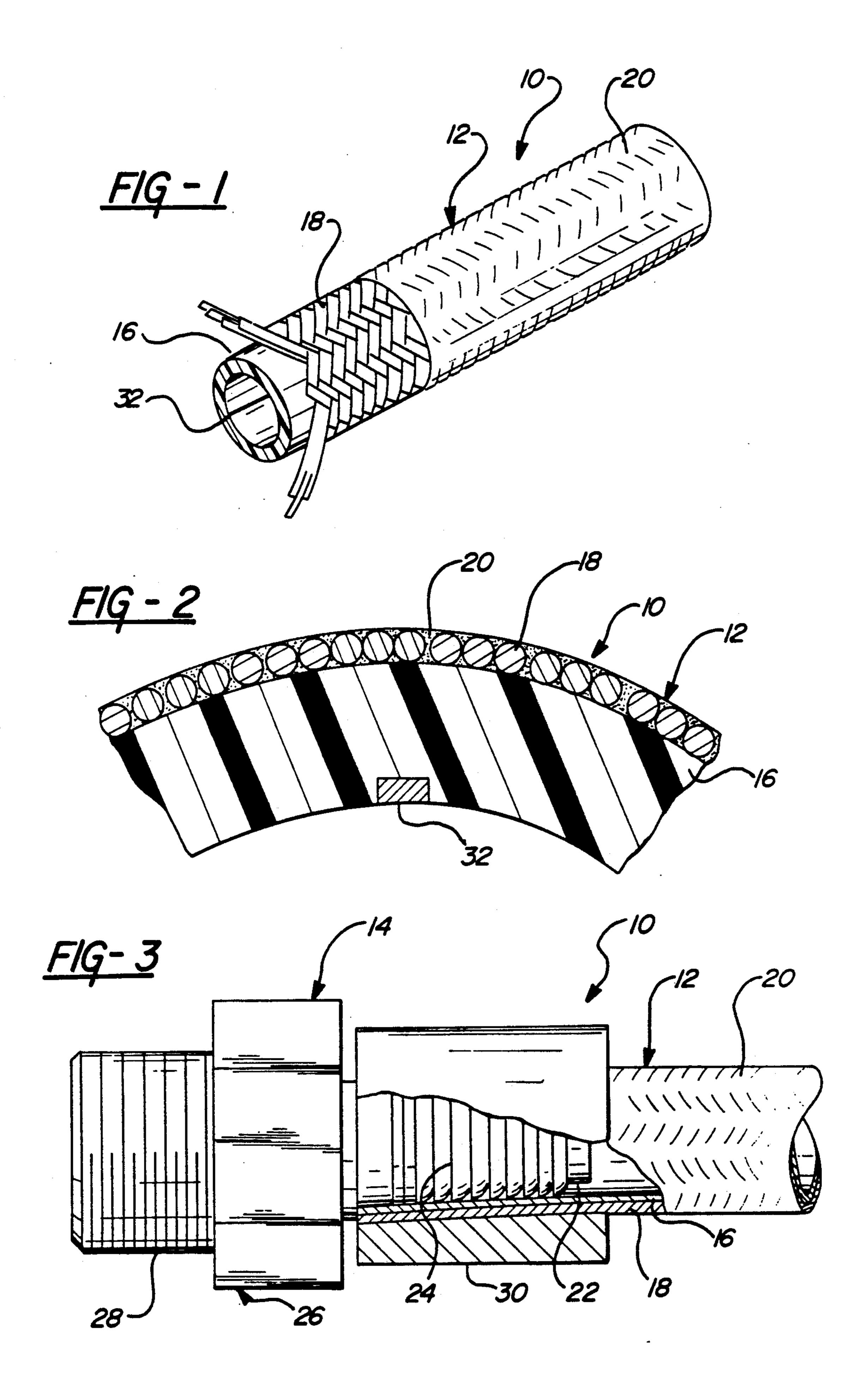
cordingly, due to exposure to frictional movement, the hose assembly must be resistant to abrasion.
