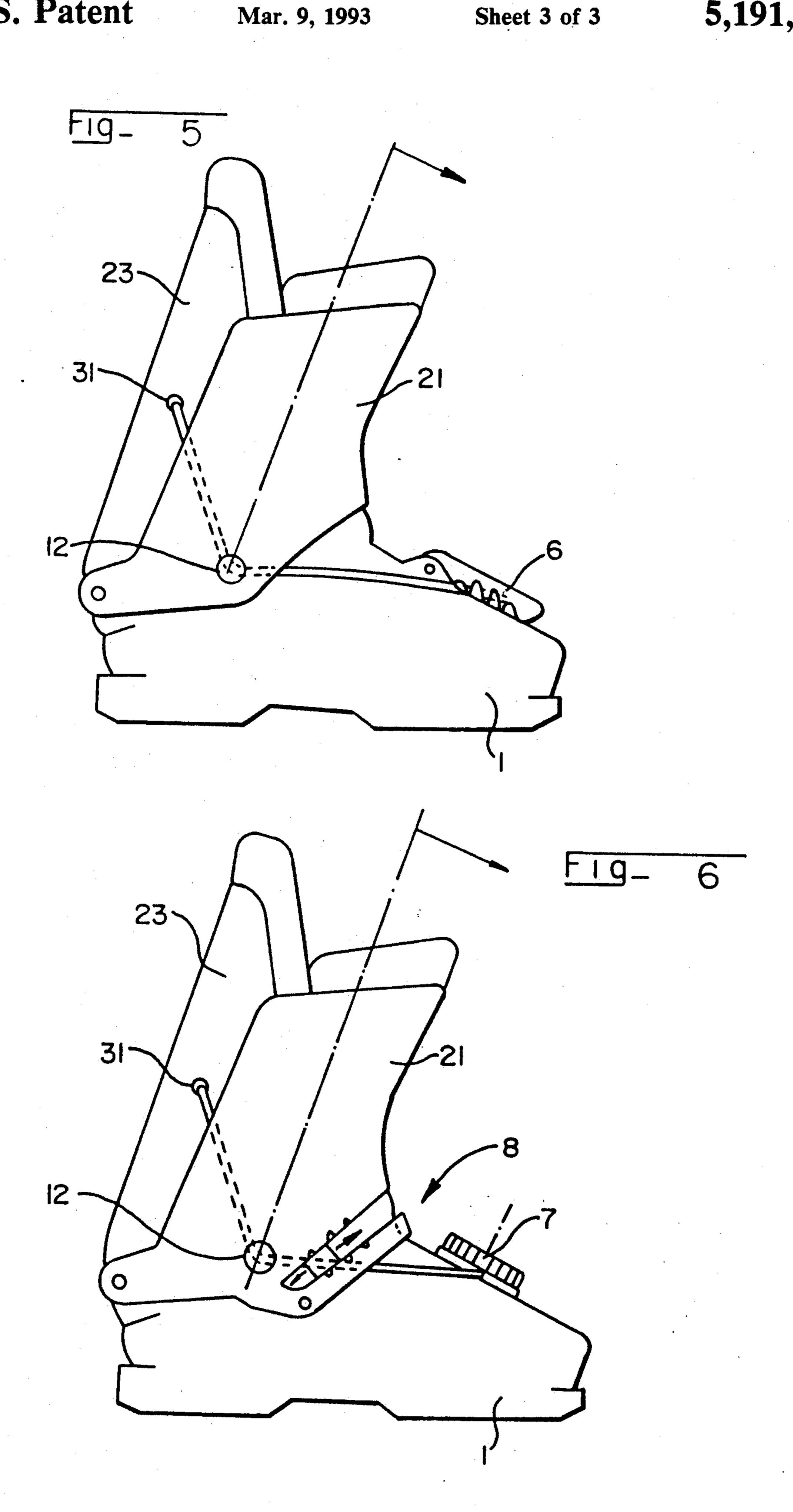
SKI BOOT HAVING A REAR SPOILER, A FRONT CUFF AND A LINKAGE, WHEREIN THE LINKAGE EXTENDS FROM LATERAL SPACED LOCATIONS AT THE SIDES OF THE BOOT TO ANCHORAGE POINTS
