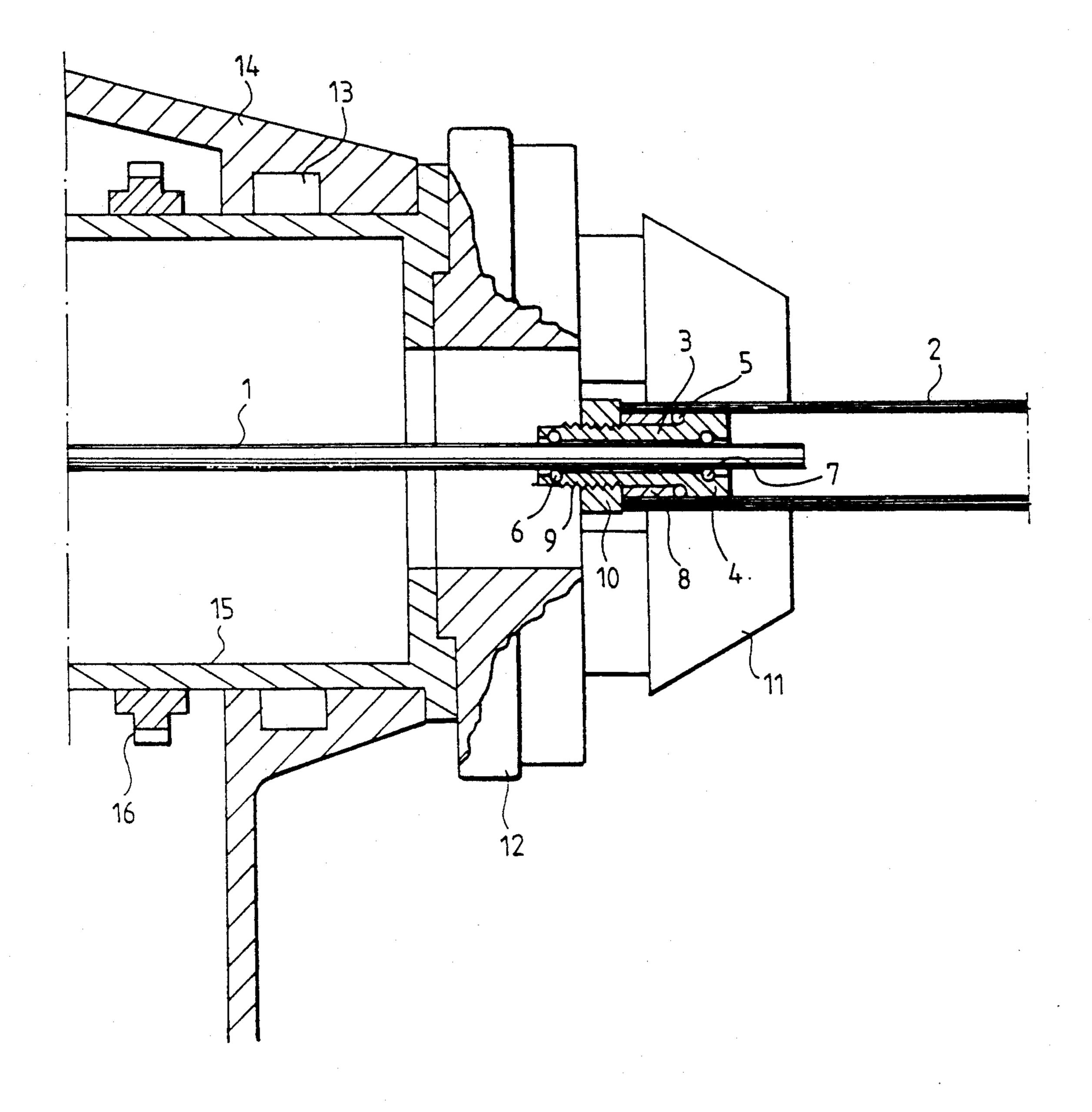
tor of the invention and a silica pipe when fitted in a lathe rotating the silica tube.
