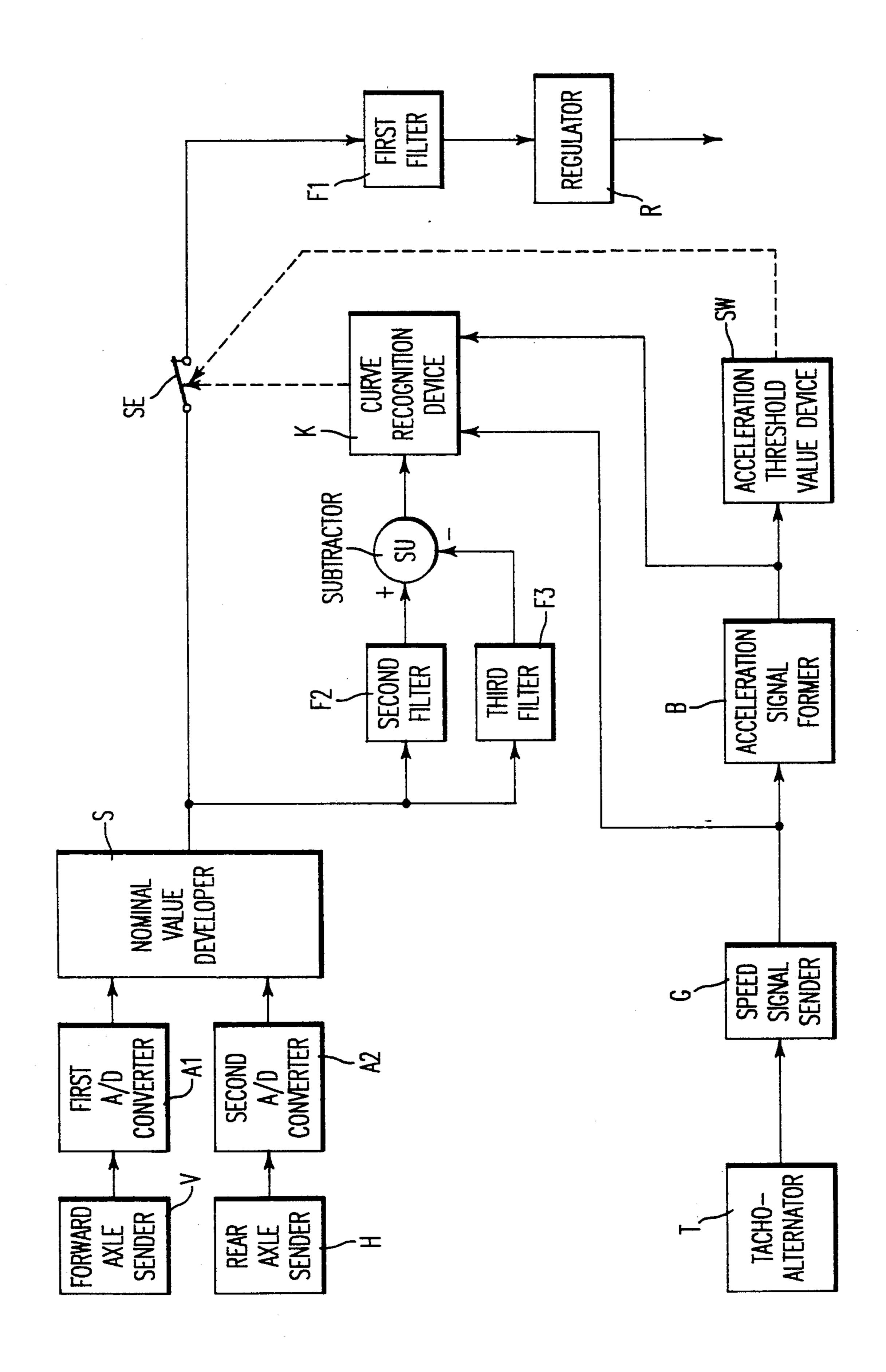
METHOD AND APPARATUS TO REGULATE ILLUMINATION RANGE OF A MOTOR VEHICLE
