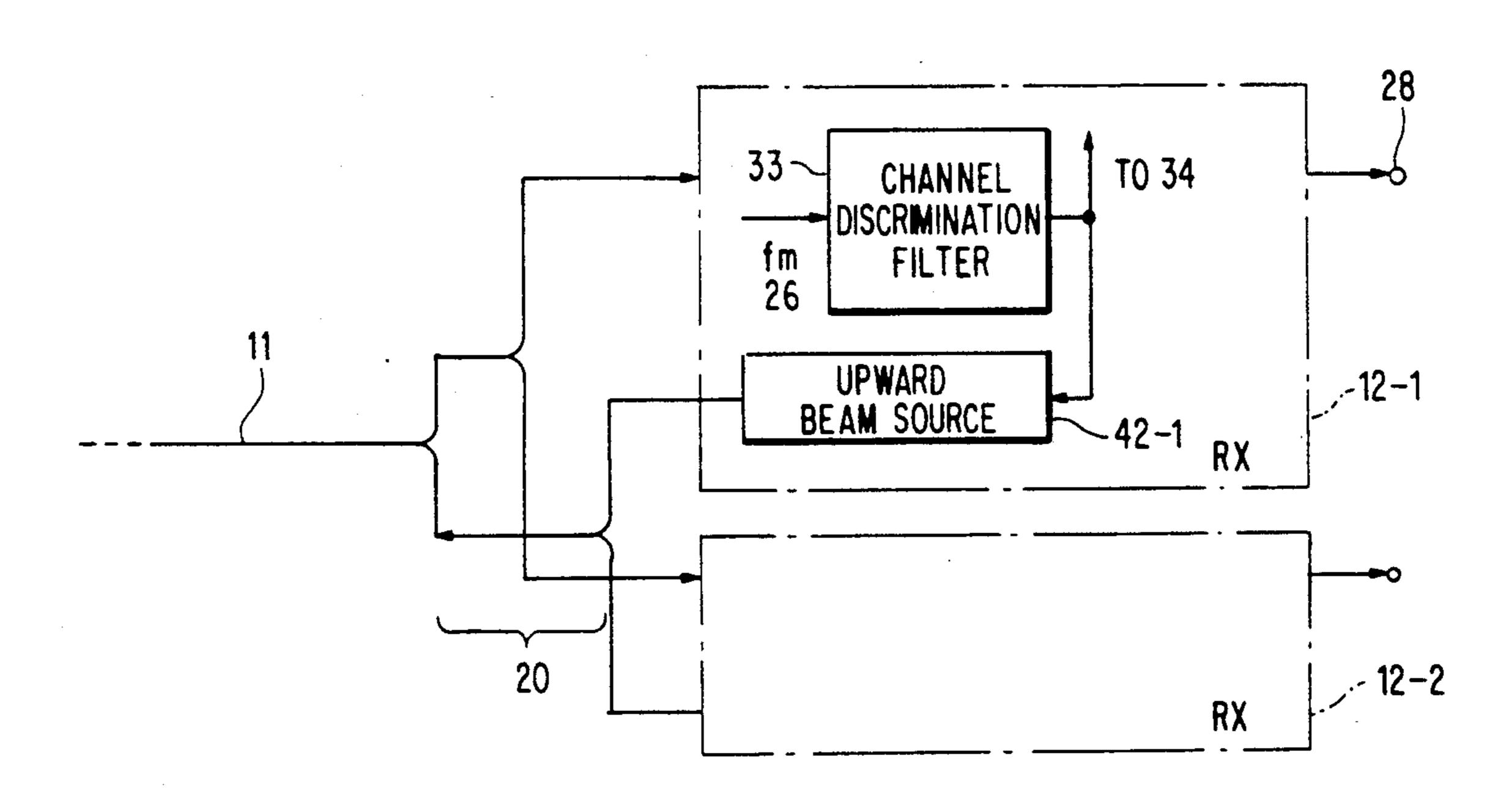
WDM OPTICAL COMMUNICATION WHEREIN OPTICAL BEAMS ARE MODULATED BY CHANNEL DISCRIMINATION SIGNALS OF DIFFERENT FREQUENCIES BEFORE BY DATA SIGNALS
