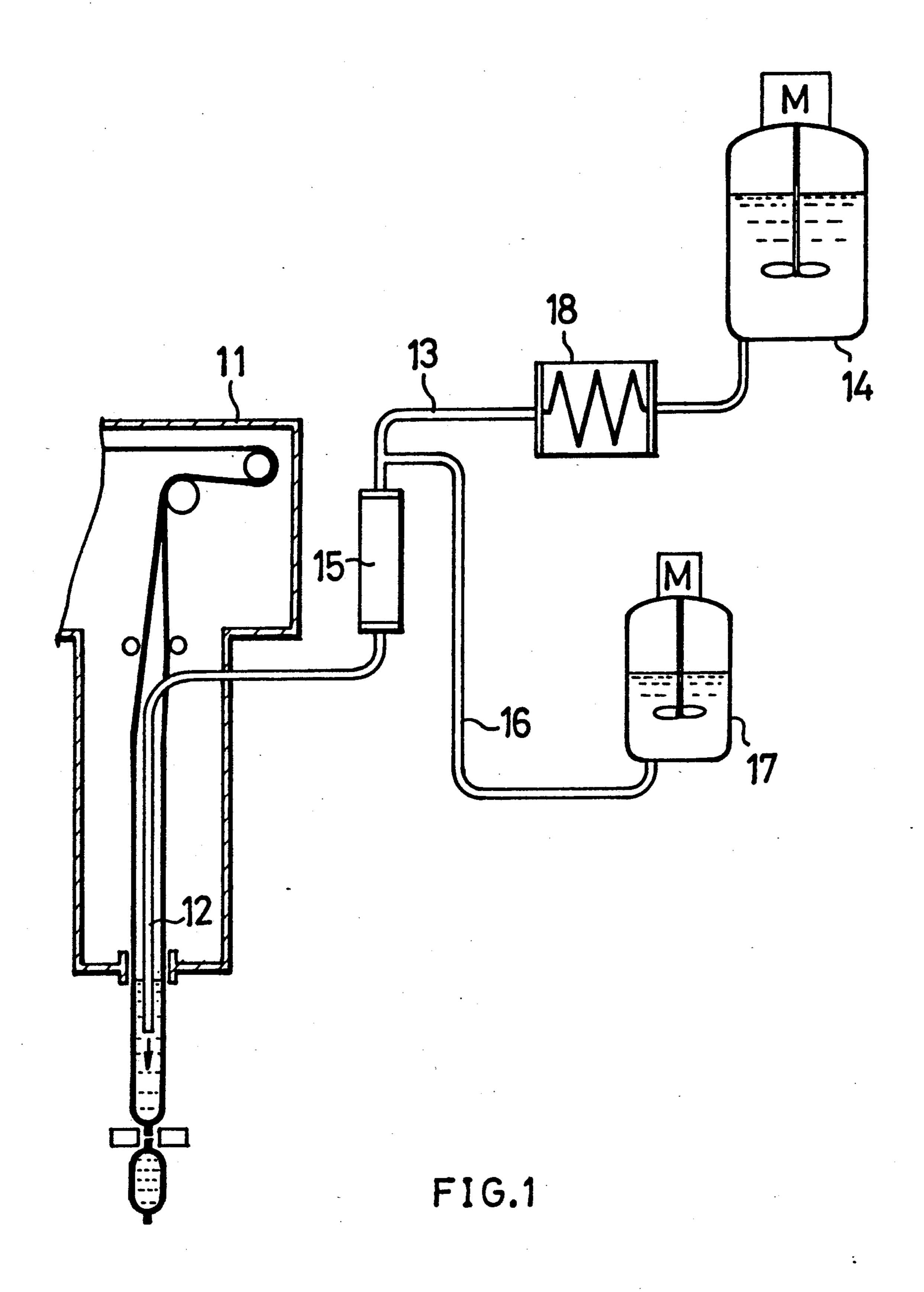
and connected to the mixer 15 by a secondary pipe 16, and a preheating heat exchanger 18 provided on the primary pipe 13 and positioned between the milk tank 14 and the mixer 15.
