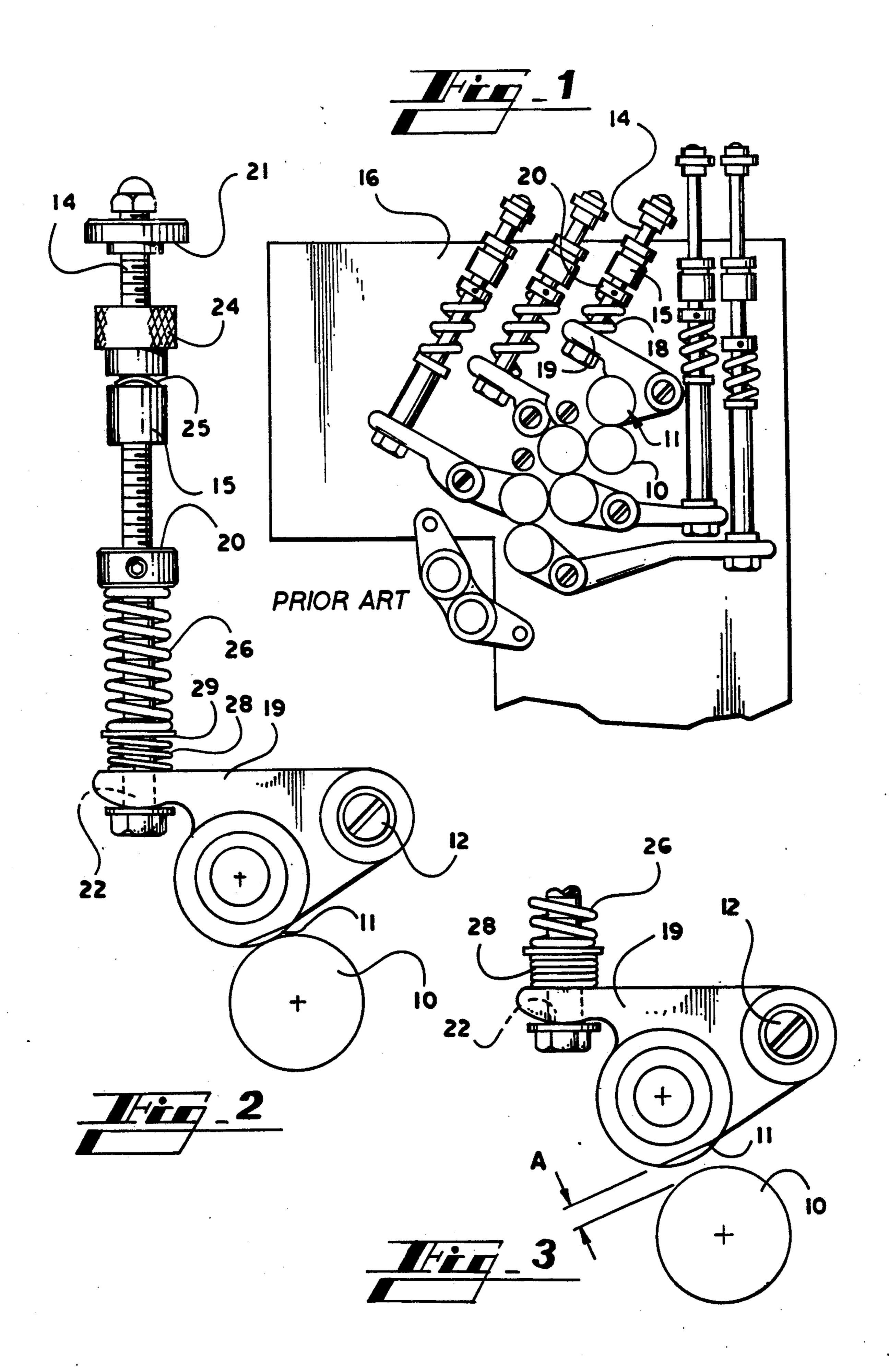
prior art gap adjusting means for the gaps at the nips of the rollers;
