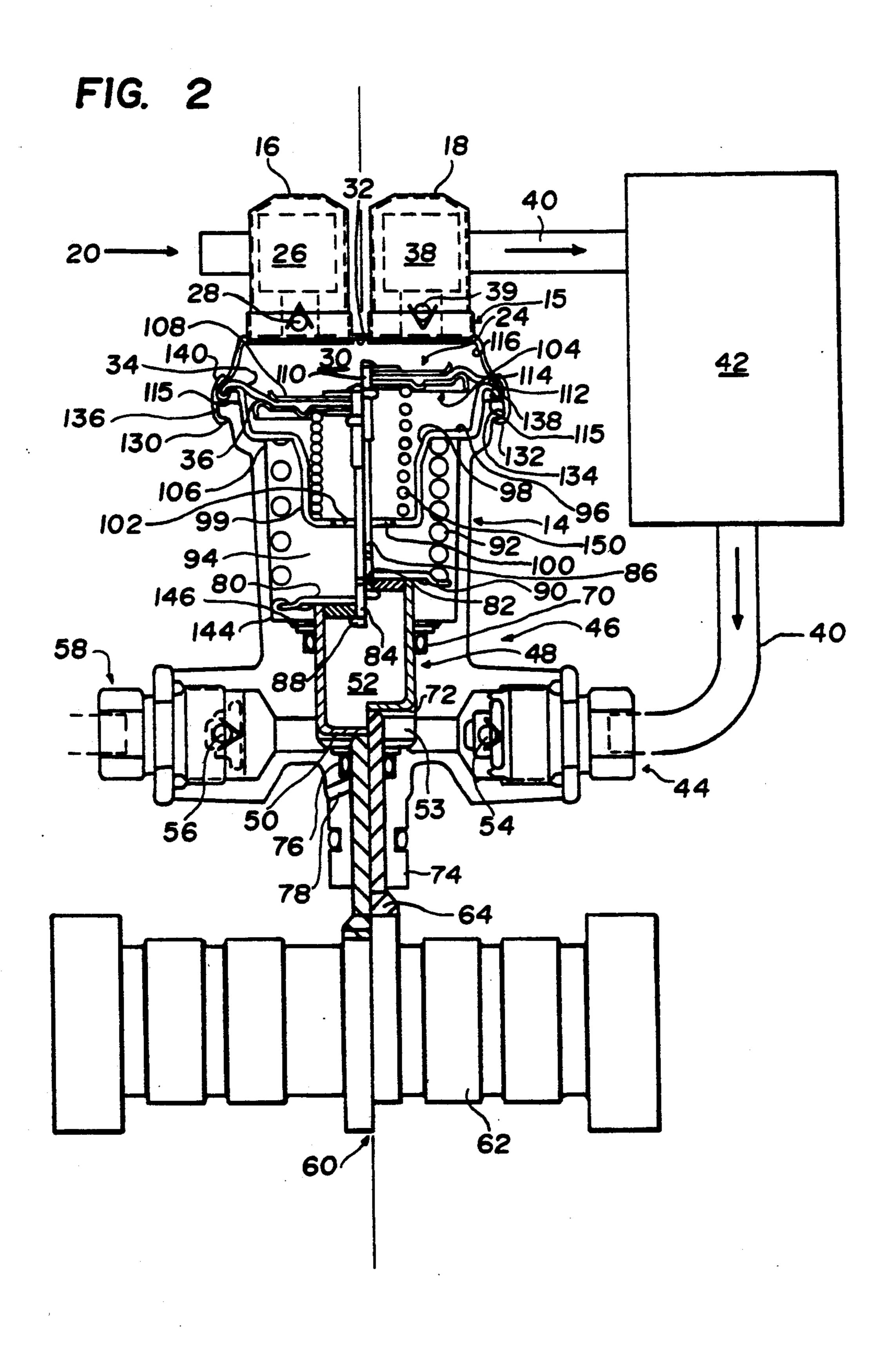
the diaphragm through the stem against the action of its biasing spring to fill the first chamber during the pumping stroke of the piston pump.
