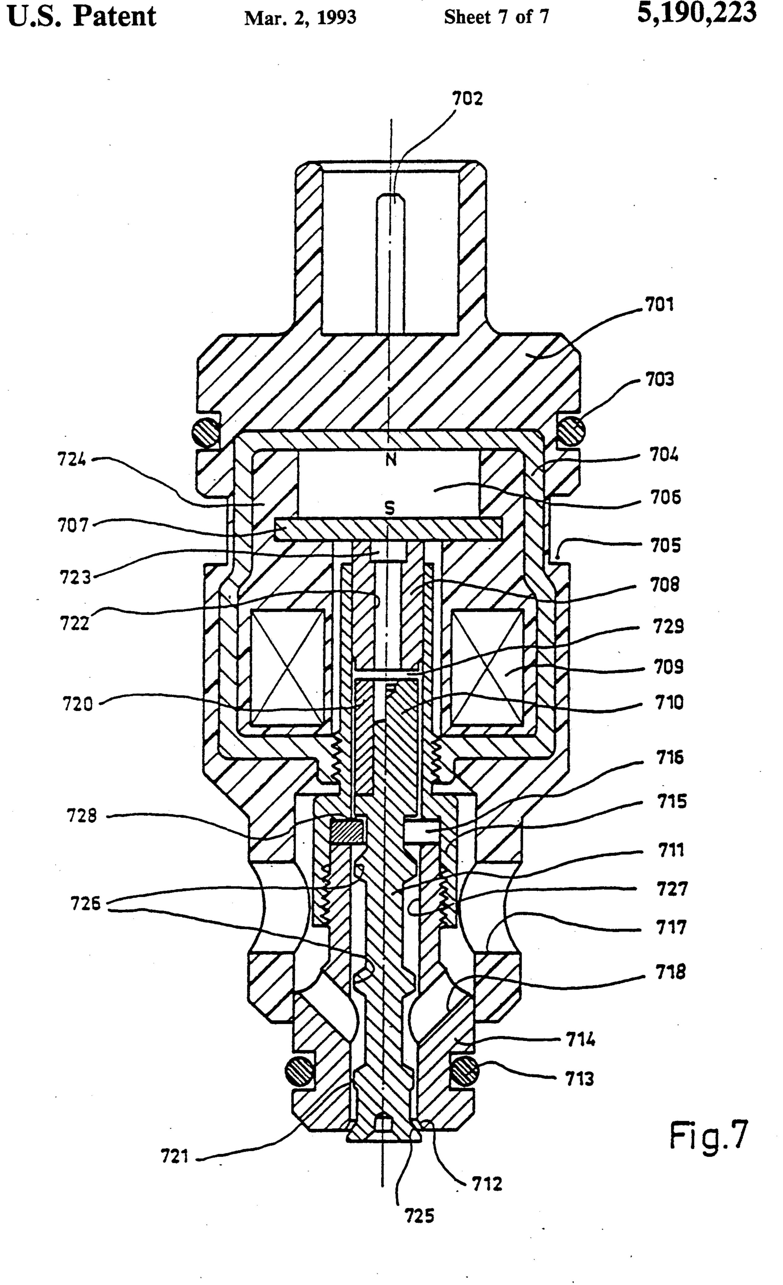
ELECTROMAGNETIC FUEL INJECTOR WITH CARTRIDGE EMBODIMENT
