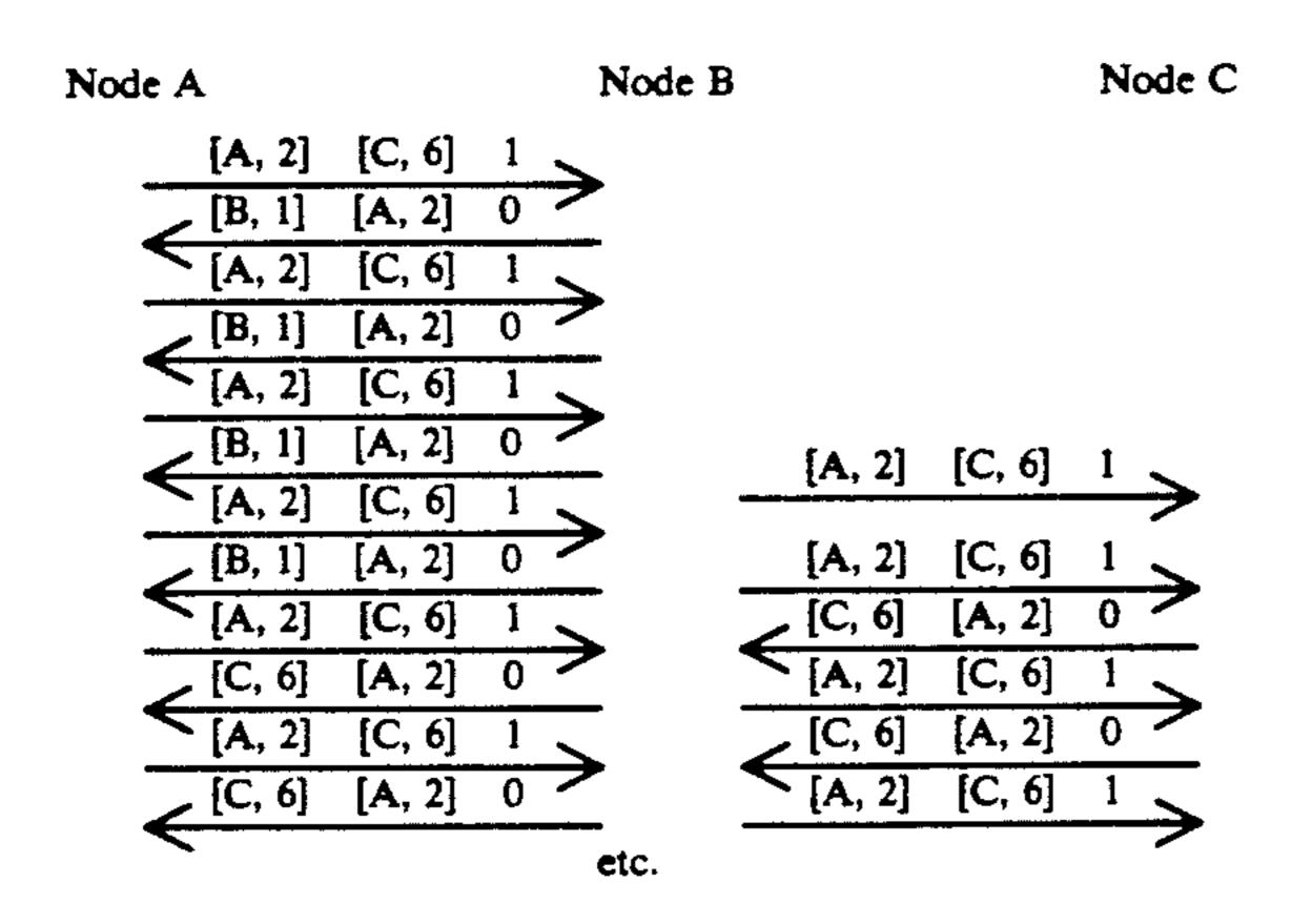
The above table does not represent an exact timing diagram, but only shows the identifications that are sent
