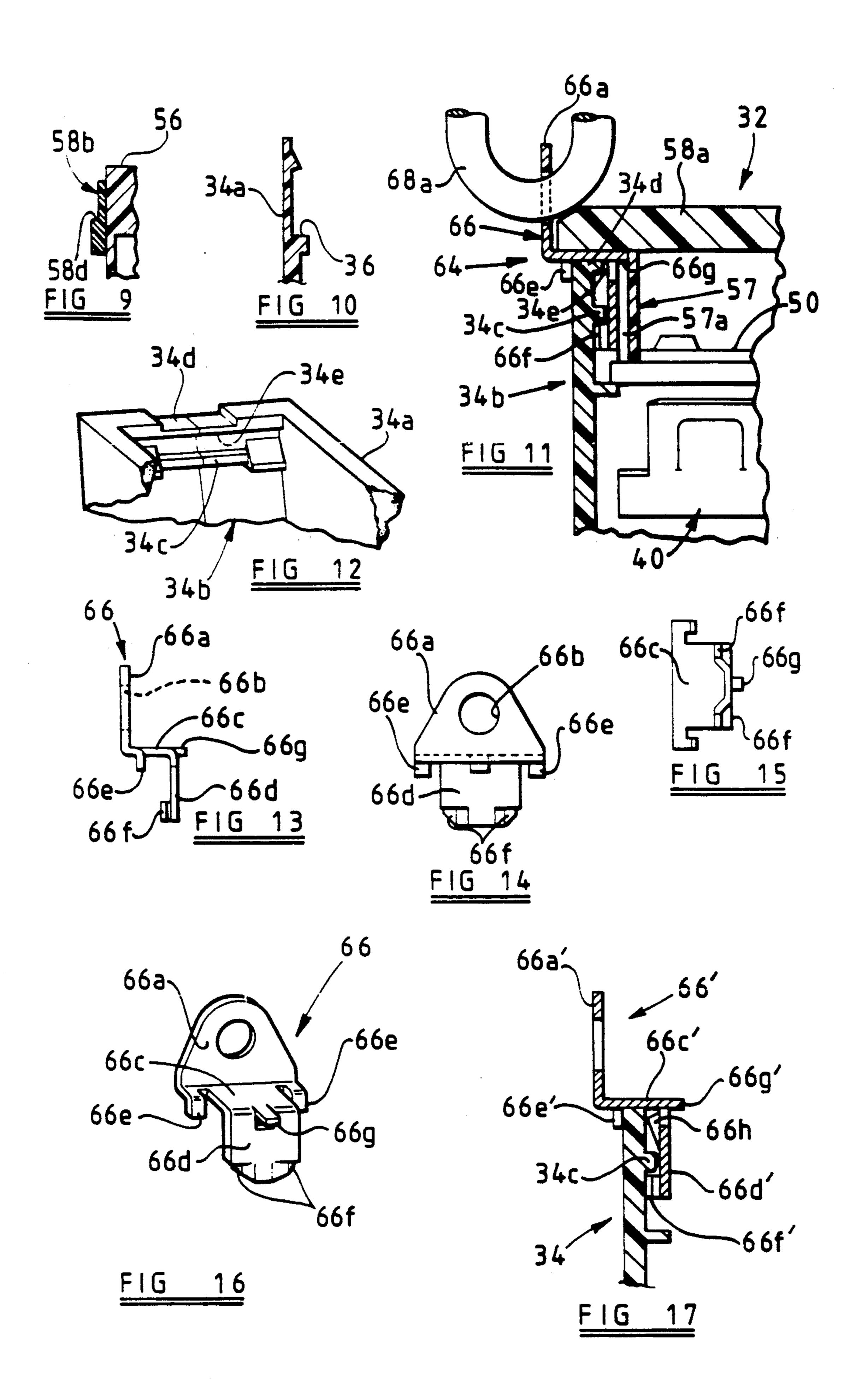
In the form of locking device consisting of a padlock and a locking clip, the clip may be retentively secured to the apparatus. In a distinctive form, both the padlock and the clip as well are removable from the electrical
