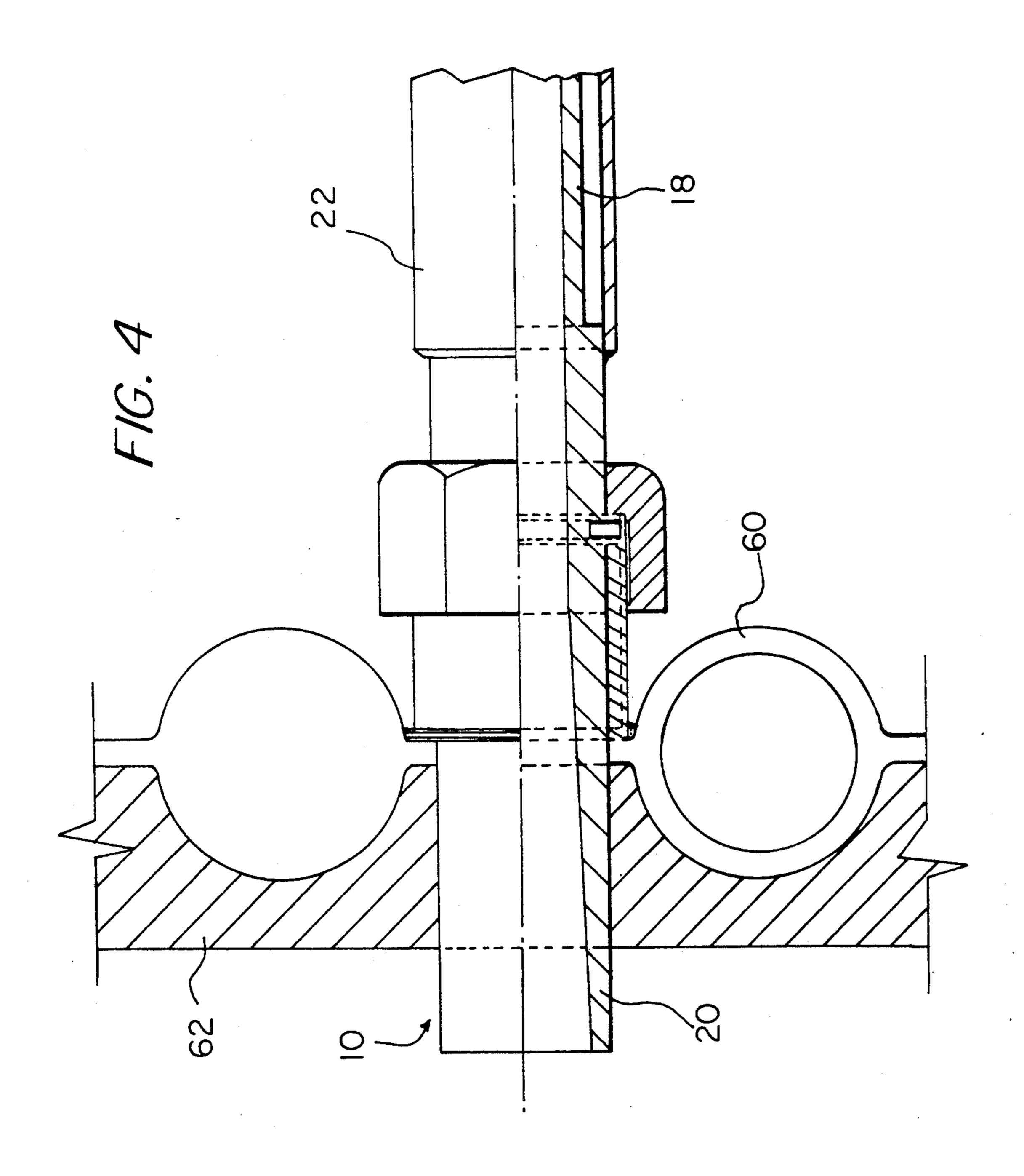
DEVICE FOR INJECTING SLUDGE INTO AN INCINERATOR
