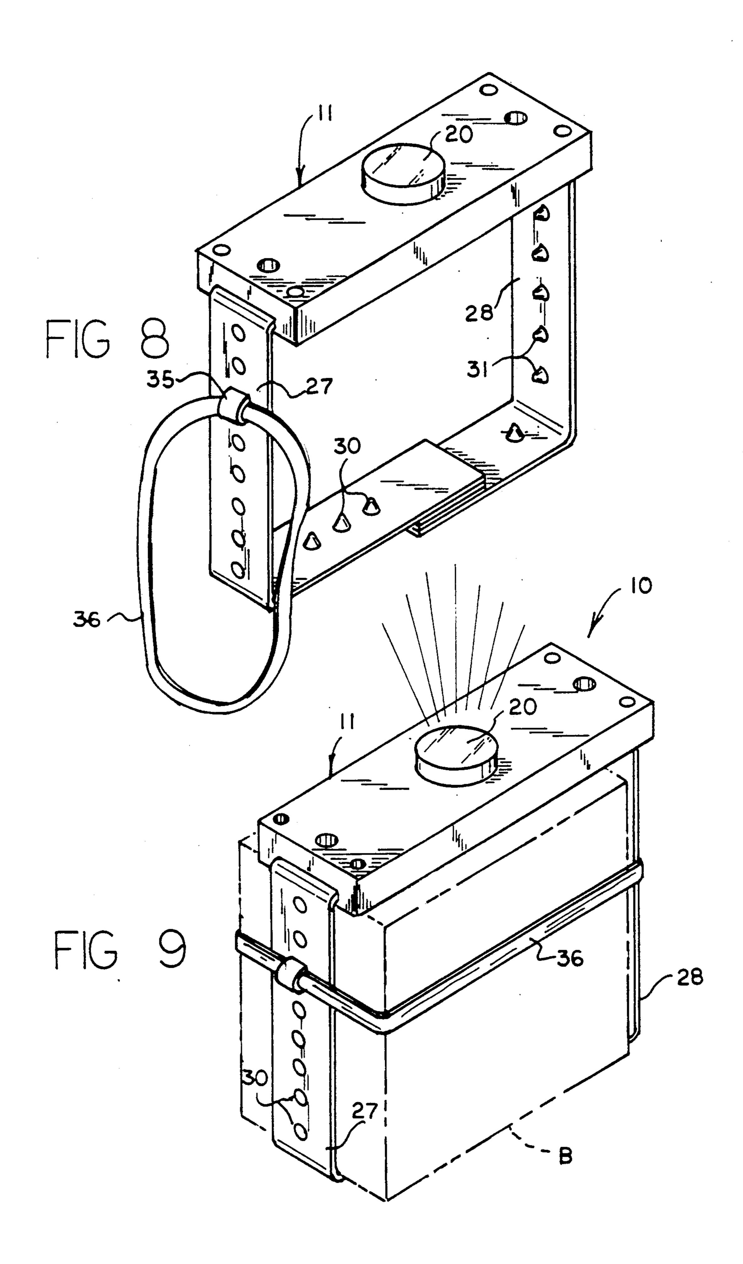
BATTERY DISCHARGE APPARATUS
