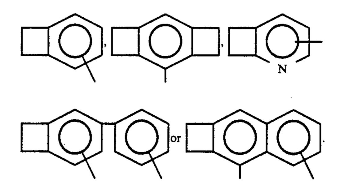
The 'side ring' of an arylcyclobutene contains two carbon atoms not in the aromatic ring that are connected to adjacent carbon atoms on the same aryl ring, the bond between said carbon atoms and the two bonds between the carbon atoms and the aryl ring.
