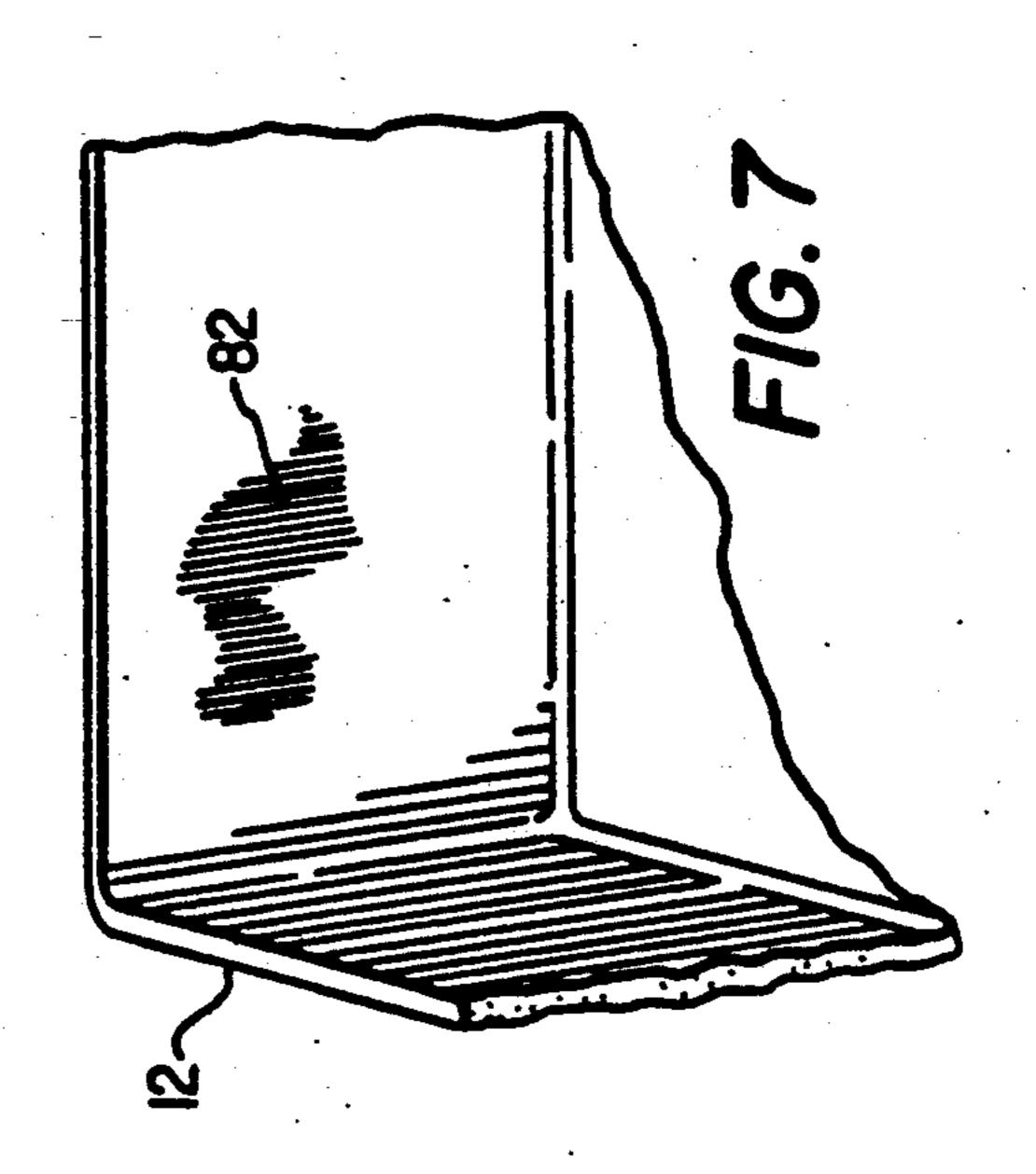
In addition, the condensate increases the possibility for rusting and other deterioration of the metal instruments in the container.
