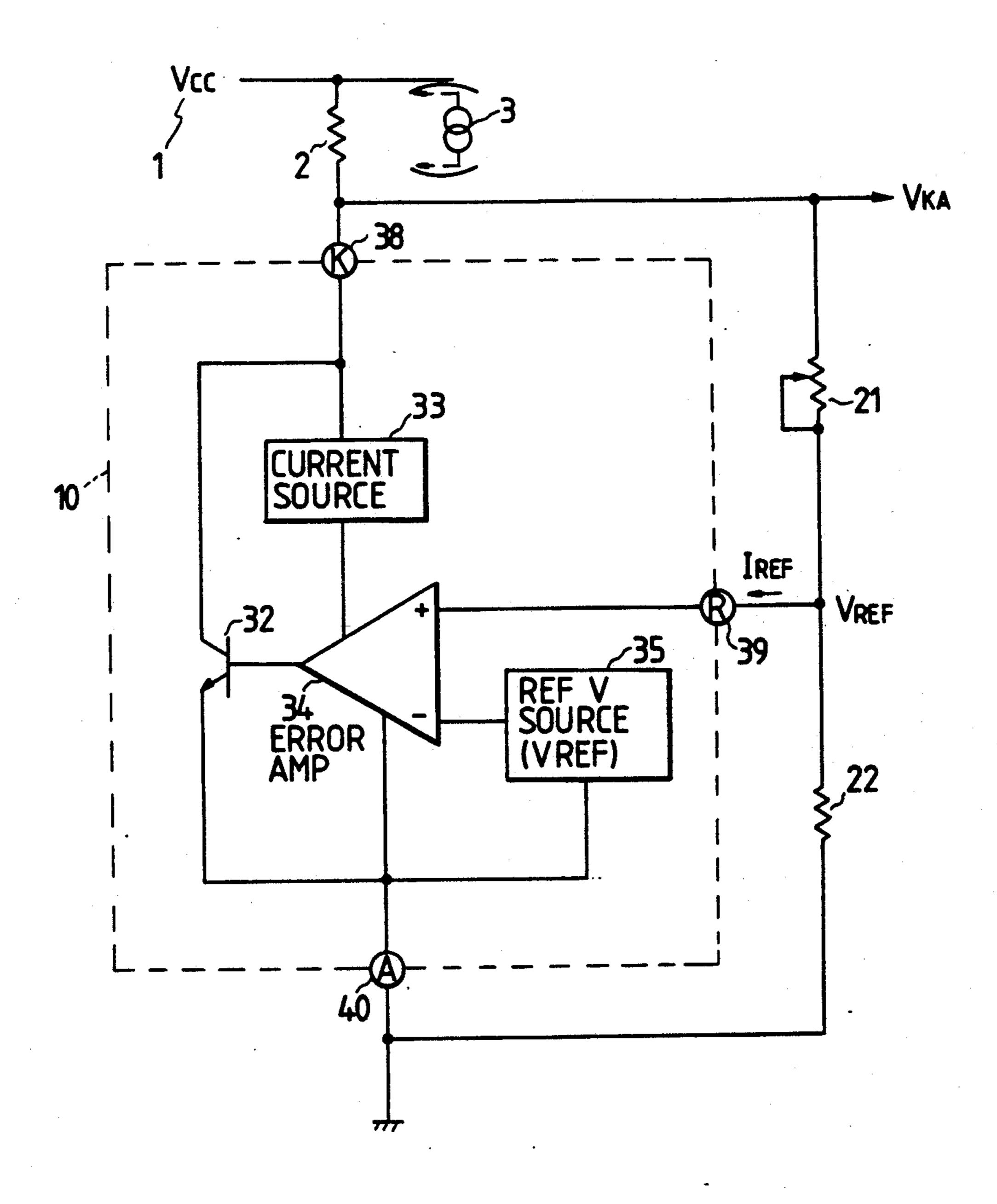
$$V_{KA} = V_{REF} \left(1 + \frac{R21}{R22}\right) + I_{REF} \cdot R21$$
