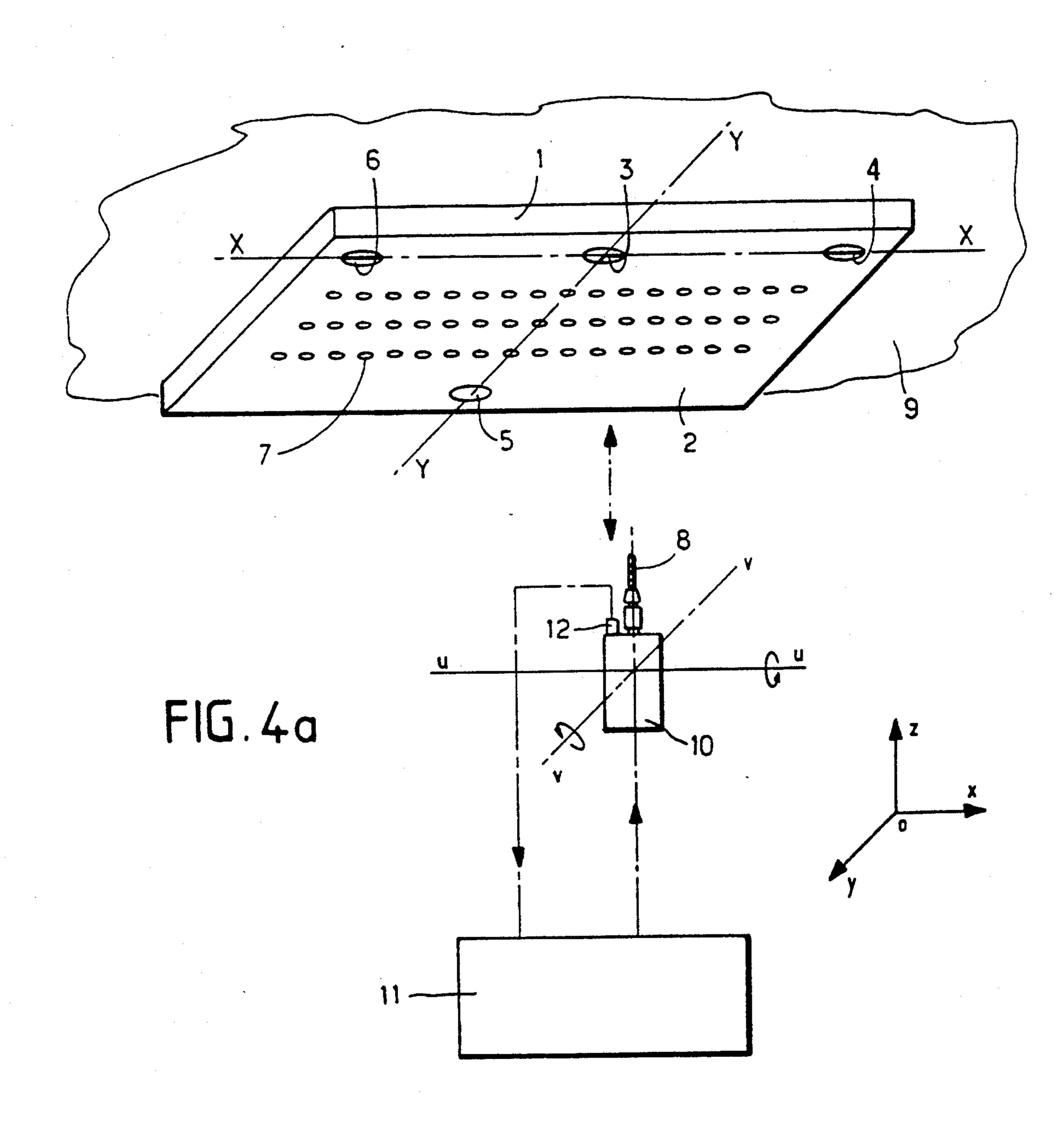
BENCHMARK DEVICE FOR A PLANE FACE, AND A MACHINING SYSTEM IMPLEMENTING IT
