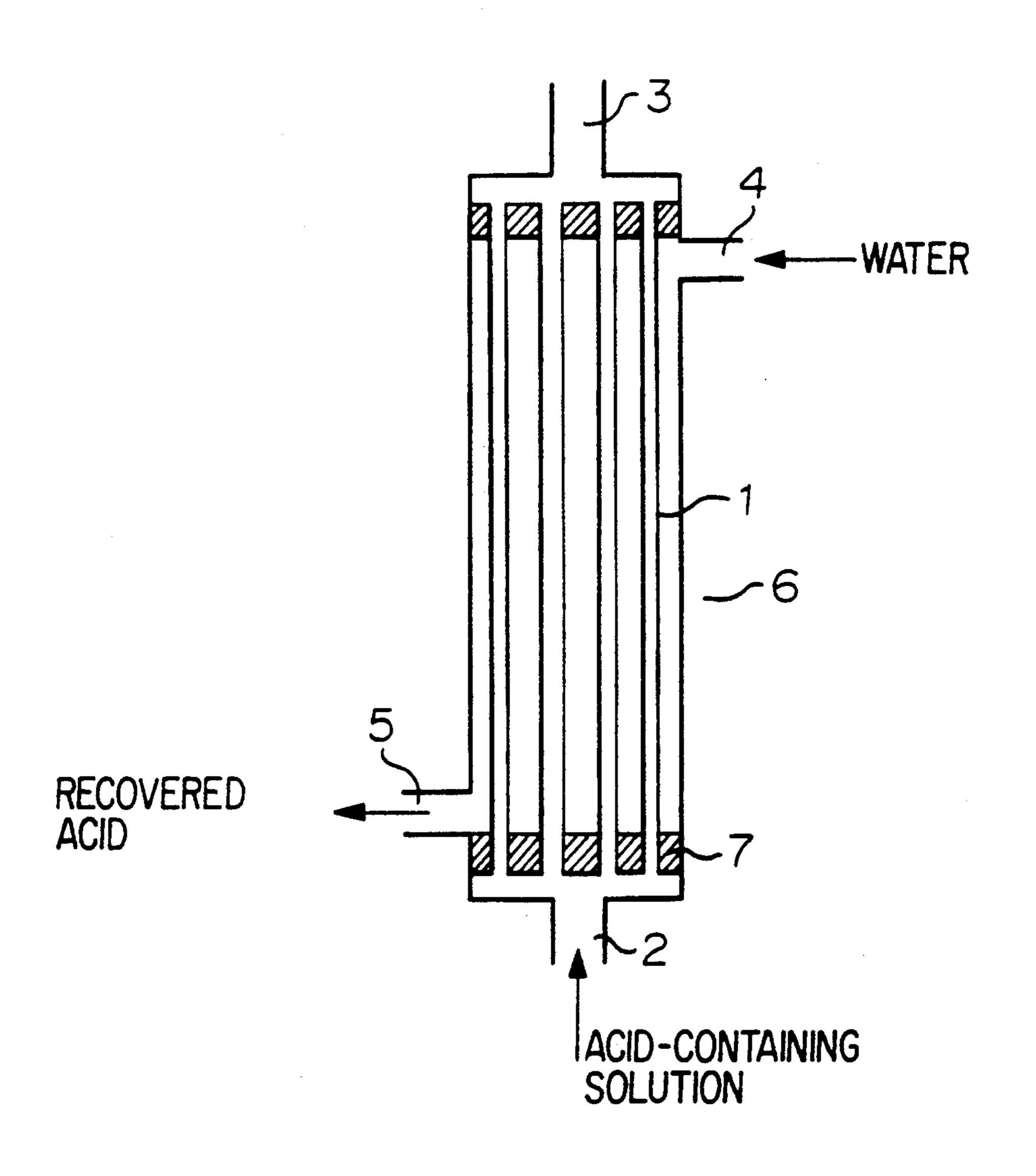
imparting ion permselectivity by introducing ion exchange groups into the membrane.
